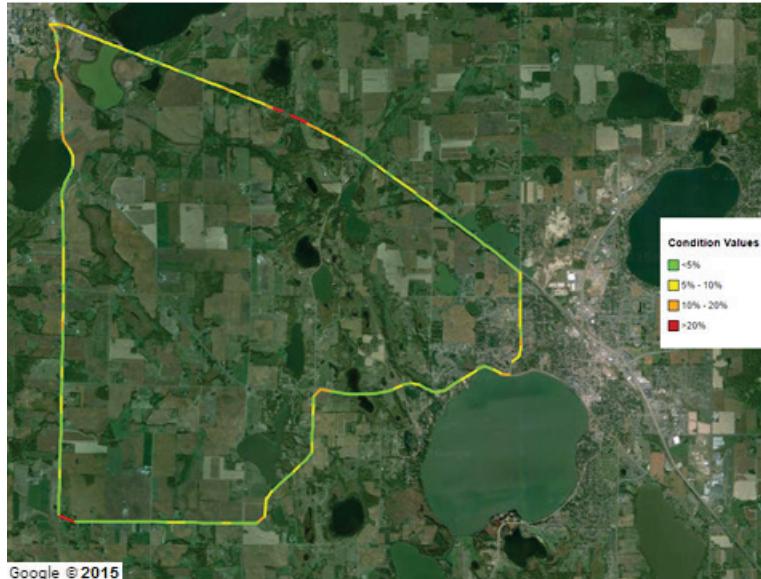
Figure 120. Map. Wright County 18-mi (29-km) loop TSD 8-inch (203.2-mm) sensor COV. (49)
