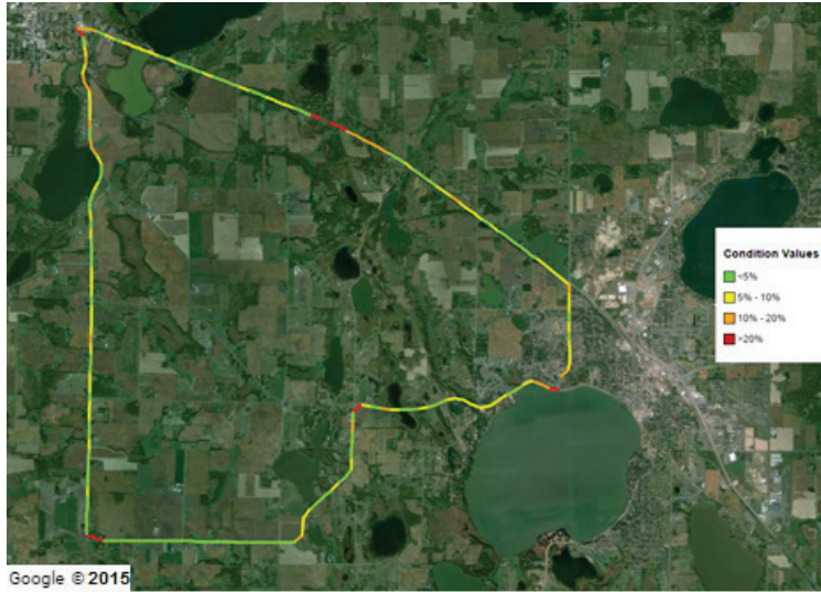
Figure 118. Map. Wright County 18-mi (29-km) loop TSD 24-inch (609.6-mm) sensor COV. (47)
