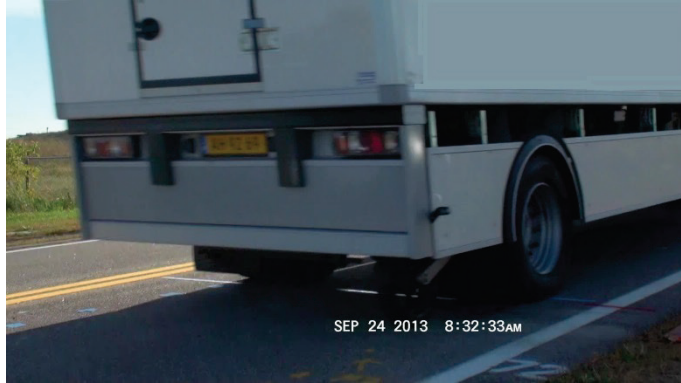
Figure 37. Photo. Sample video snapshot showing wheel location from TSD pass.
