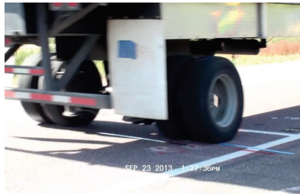
Figure 38. Photo. Sample video snapshot showing wheel location from RWD pass.
