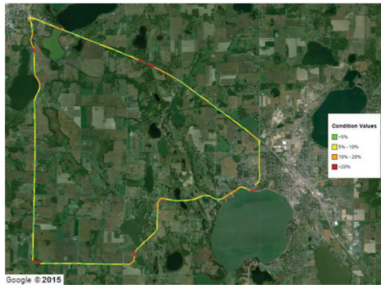
Figure 121. Map. Wright County 18-mi (29-km) loop TSD 4-inch (101.6-mm) sensor COV. (50)
