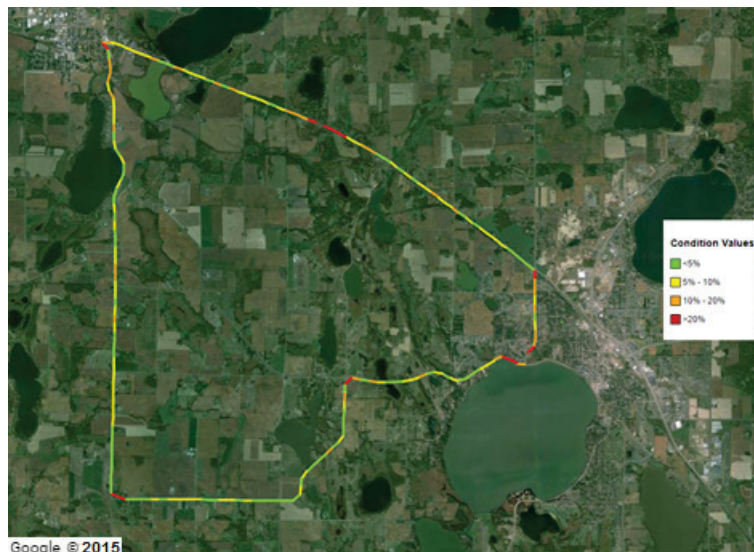
Figure 117. Map. Wright County 18-mi (29-km) loop TSD 36-inch (914.4-mm) sensor COV. (46)
