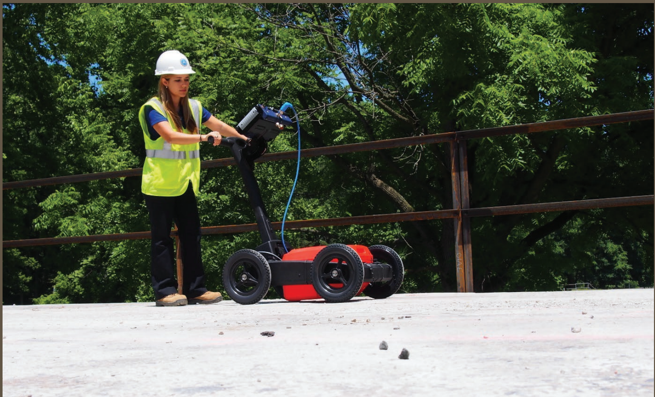
Figure 2. Data collection on a bridge deck using ground-coupled GPR.
