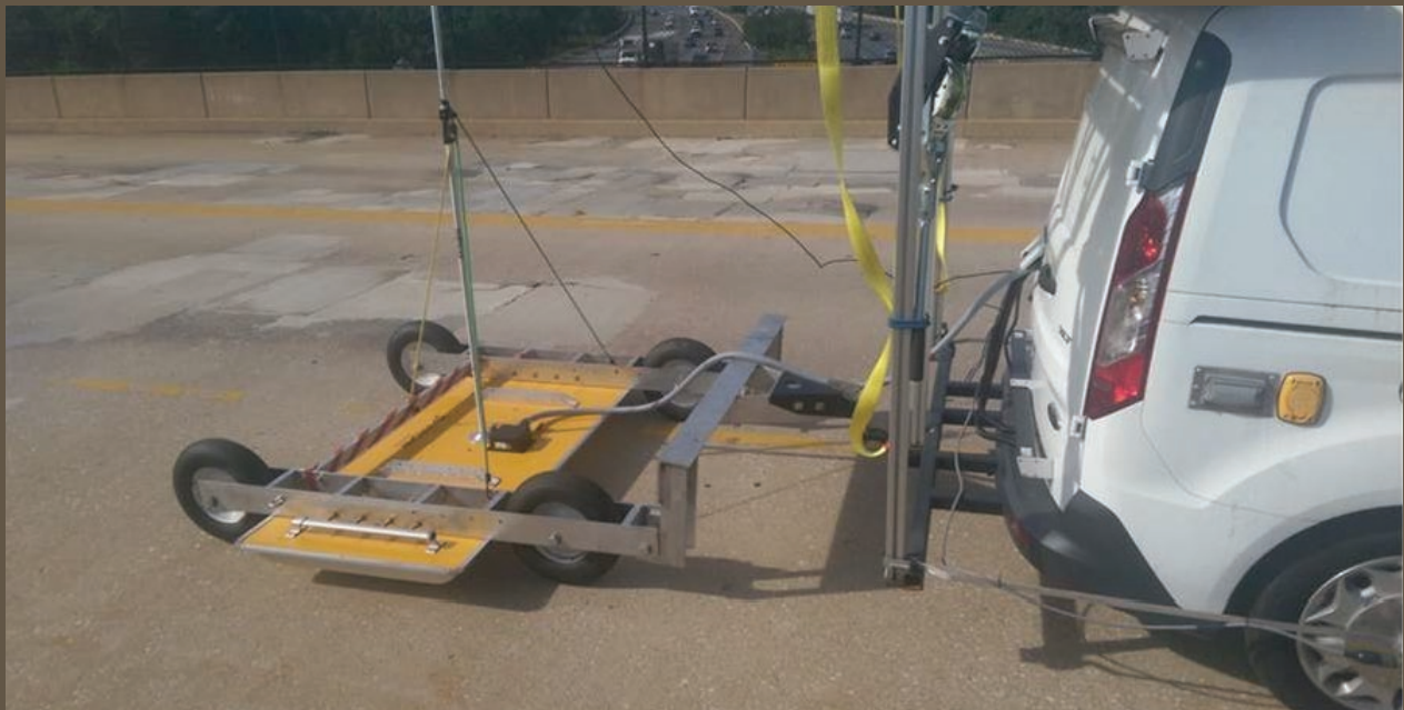
Figure 3. Data collection on a bridge deck using air-coupled GPR.
