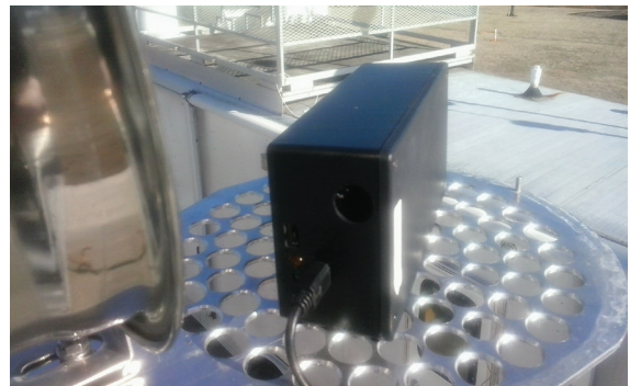
Figure 4. Deployment of a particulate matter sensor in a near-road test bed.
