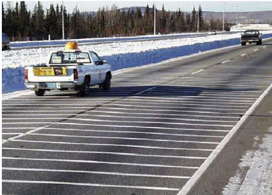
Figure 19. Photo. Transverse test deck in Alaska.
