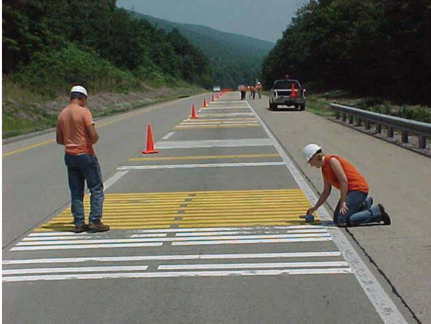
Figure 18. Photo. Typical transverse test deck.
