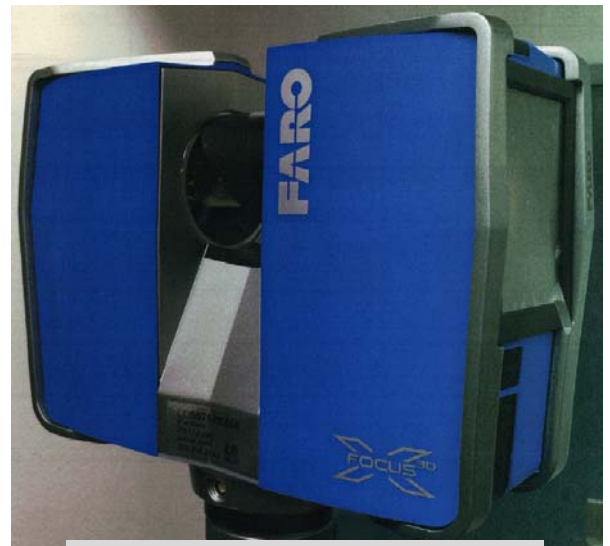
Yuma Police Department FARO 3D Laser Scanning System
