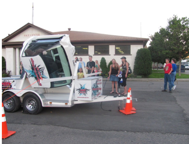
MDT Intern Michelle Erb demonstrates the effects of a rollover crash using the rollover simulator. Inside are dummies. The difference between the outcome for a buckled occupant and an unbuckled occupant—who is usually partially or fully ejected—is graphically illustrated.
