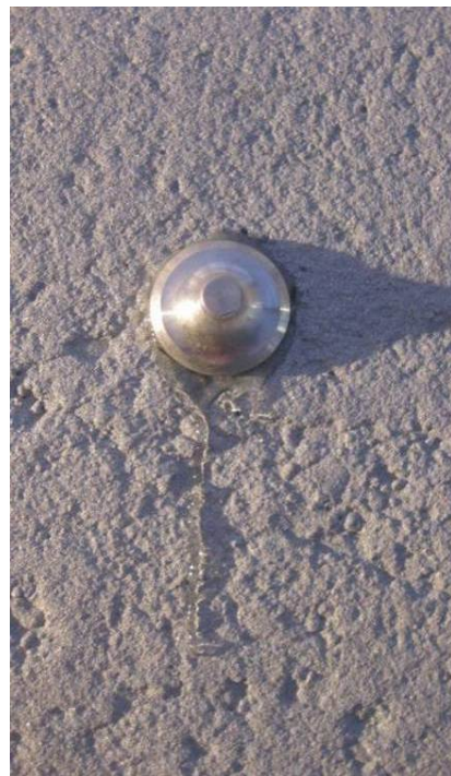
Figure 4.42: Close-up of test dolly bonded to the surface. The excess epoxy was removed before bond testing.
