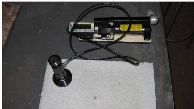
Figure 4.9: DeFlesko Posi-Test adhesion tester and metalized PCC sample ready for testing.
