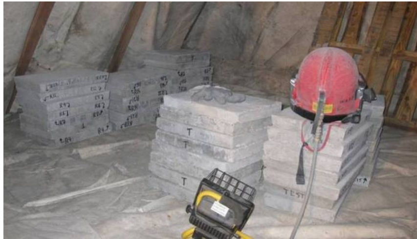
Figure 4.25: PCC and mortar samples acclimatizing in enclosure.
