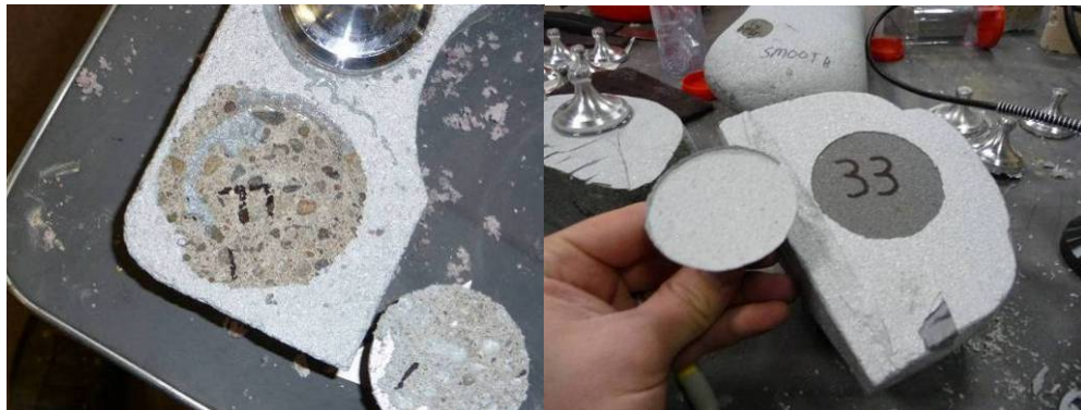
Figure 4.13: Typical NETL sample (left) and rock sample (right) after bond testing.
