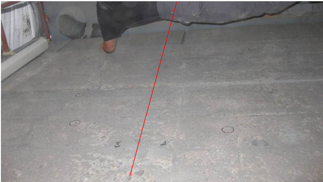
Figure 4.33: The bridge section profiled by a #8 nozzle with medium and low sand volume. Medium profile is to the left of the red line.
