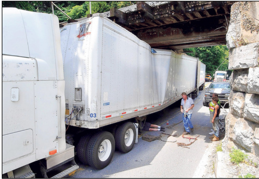
Figure 48. Photo. A Truck that Collided with the MD 75 Bridge. (7)
