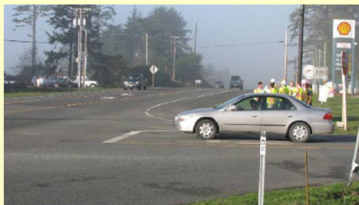
View of Indian Road intersection looking north. Photo shows the relatively wide cross-section and limited sight distance to the north due to the crest vertical curve.
