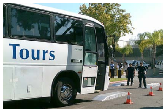
FMCSA inspector directs a bus onto ramps for a Level I (complete vehicle and driver) inspection at Otay Mesa, CA.
