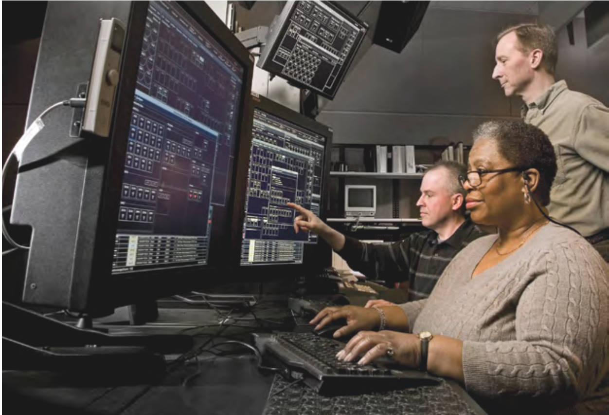
ERAM (En Route Automation Modernization) system monitor and control consoles. Photo: FAA.
