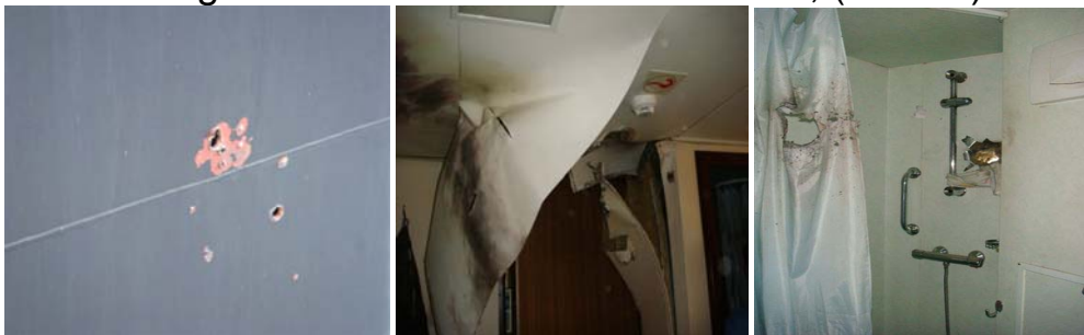
Damage caused by RPG's to Maersk Regensburg
