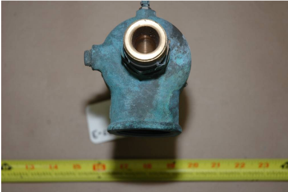
Figure 29: Shows PRD identified as 08H127-3
