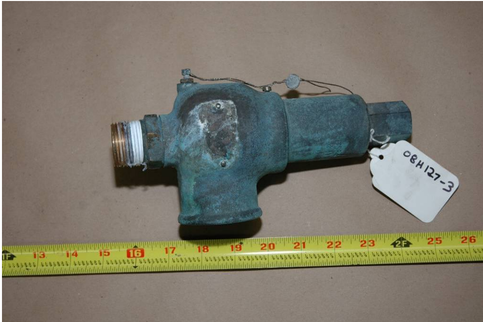
Figure 27: Shows PRD identified as 08H127-3
