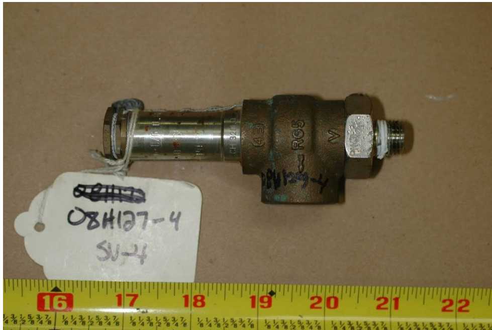
Figure 51: Shows PRD identified as 08H127-4
