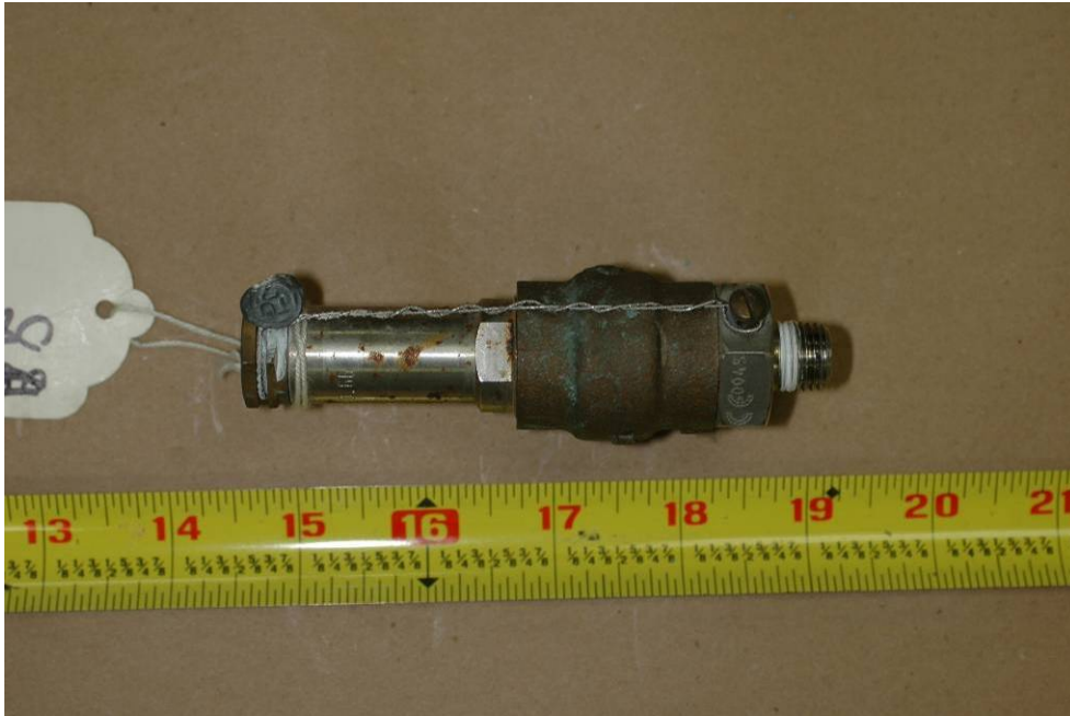
Figure 55: Shows PRD identified as 08H127-4
