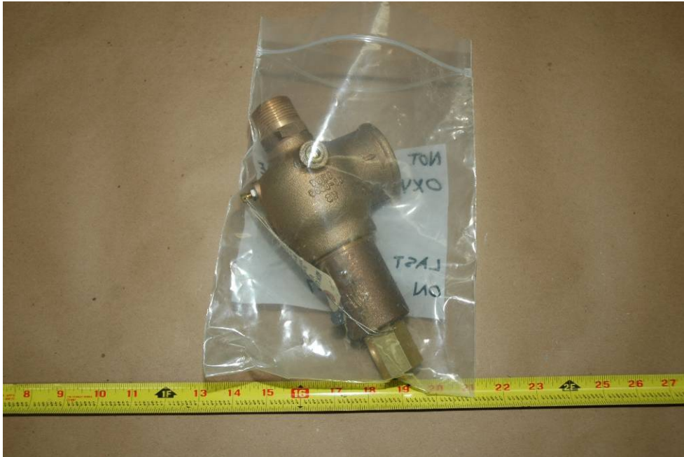
Figure 37: Shows the as received PRD identified as 08H127-Exemplar
