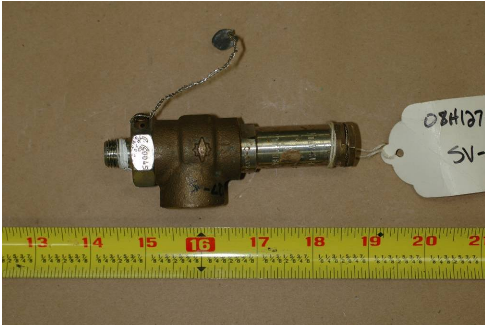
Figure 65: Shows PRD identified as 08H127-5
