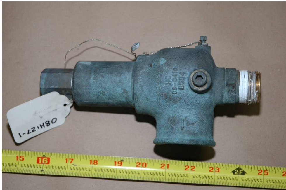
Figure 4: Shows PRD identified as 08H127-1
