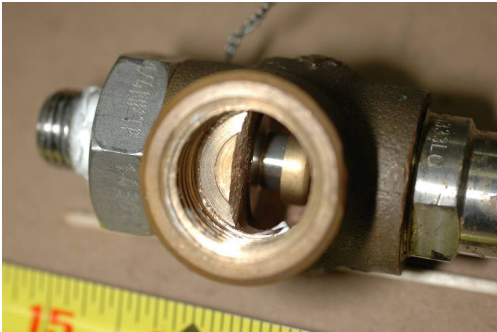
Figure 70: Shows PRD identified as 08H127-5
