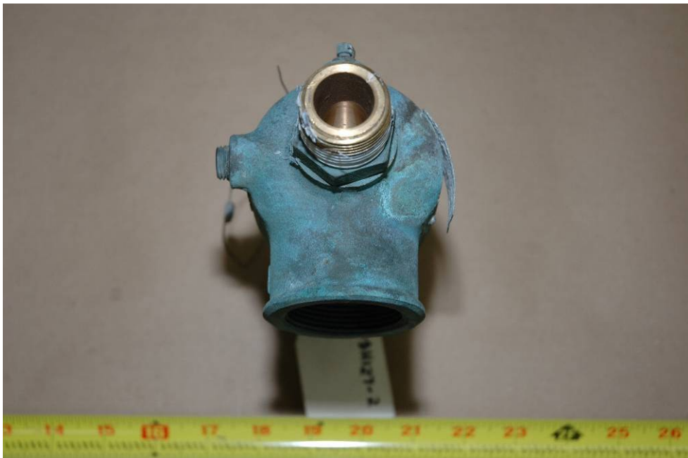
Figure 18: Shows PRD identified as 08H127-2
