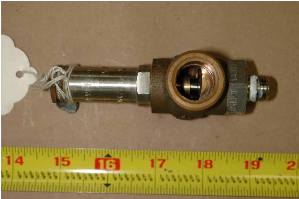
Figure 56: Shows PRD identified as 08H127-4
