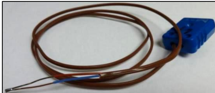
Figure A2. Thermocouple fabricated by LOGSA
