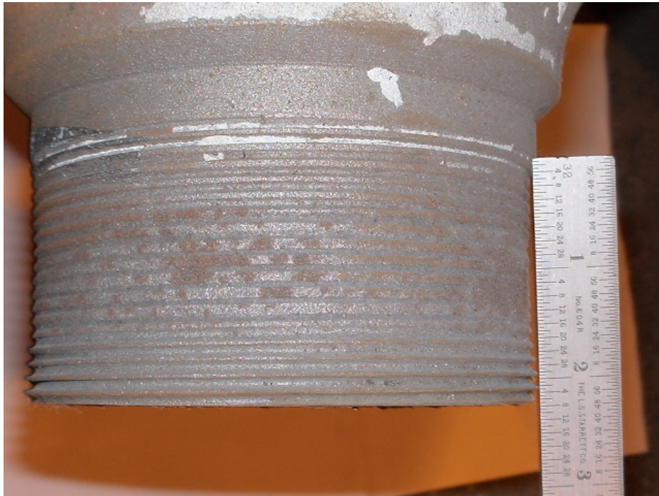
Figure 2 - Visualization of Thread Wear Using a Straightedge (Note the gap between the straightedge and the peak of the damaged threads)
