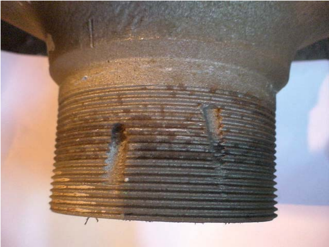
Figure 4 - Example of Isolated Damage from Anti-rotation Pins
