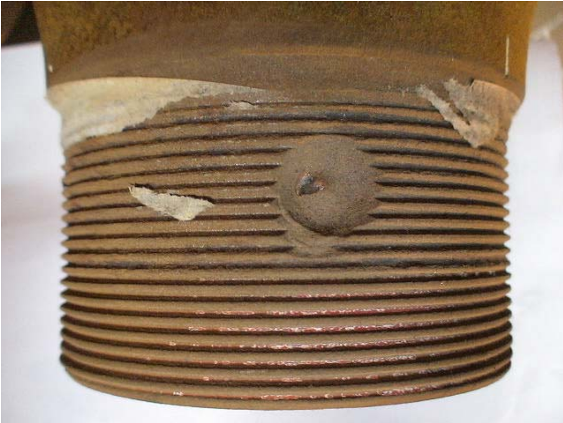
Figure 5 - Example of Isolated damage from Setscrew
