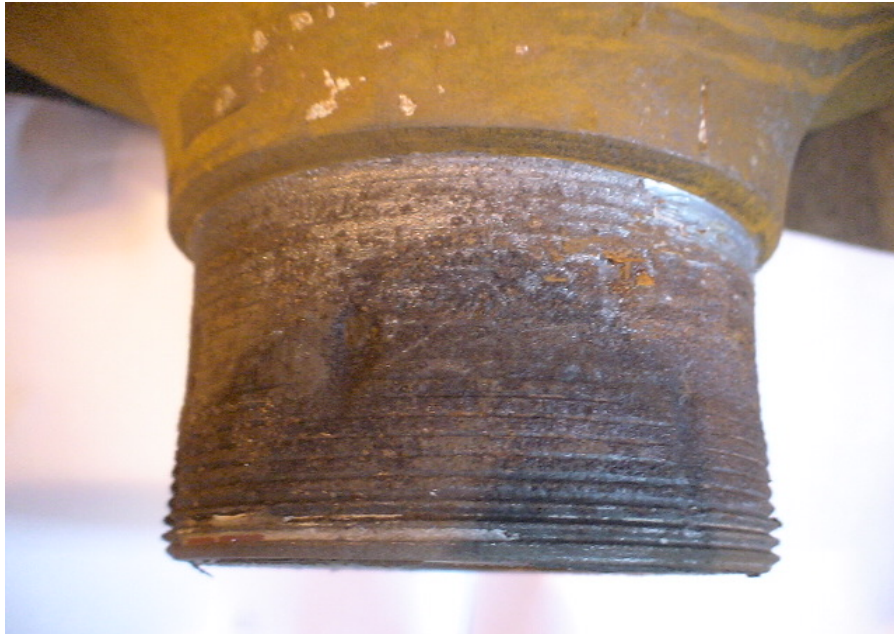
Figure 1- Example of Generalized Thread Wear
