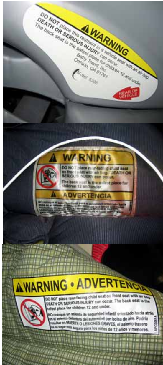
Appendix D. Example warning labels affixed the CRS A, B, C (top to bottom).
