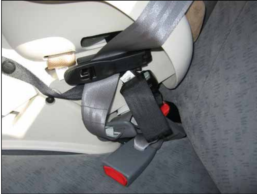
Figure 13. The lock-off on CRS D is a feature difference that contributed to seat belt routing misuse.
