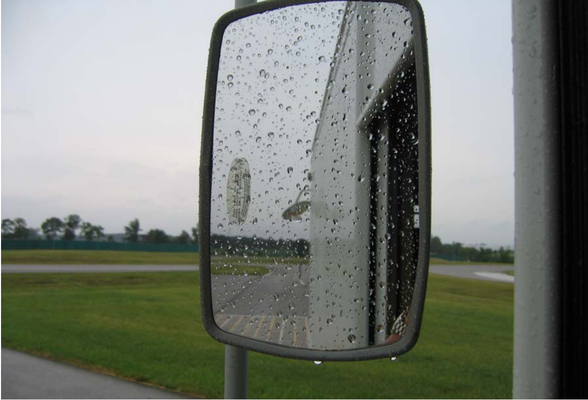
Figure 62. Driver's View of the Rear Cross-view Mirror in the Side-view Mirror During Light Rainfall
