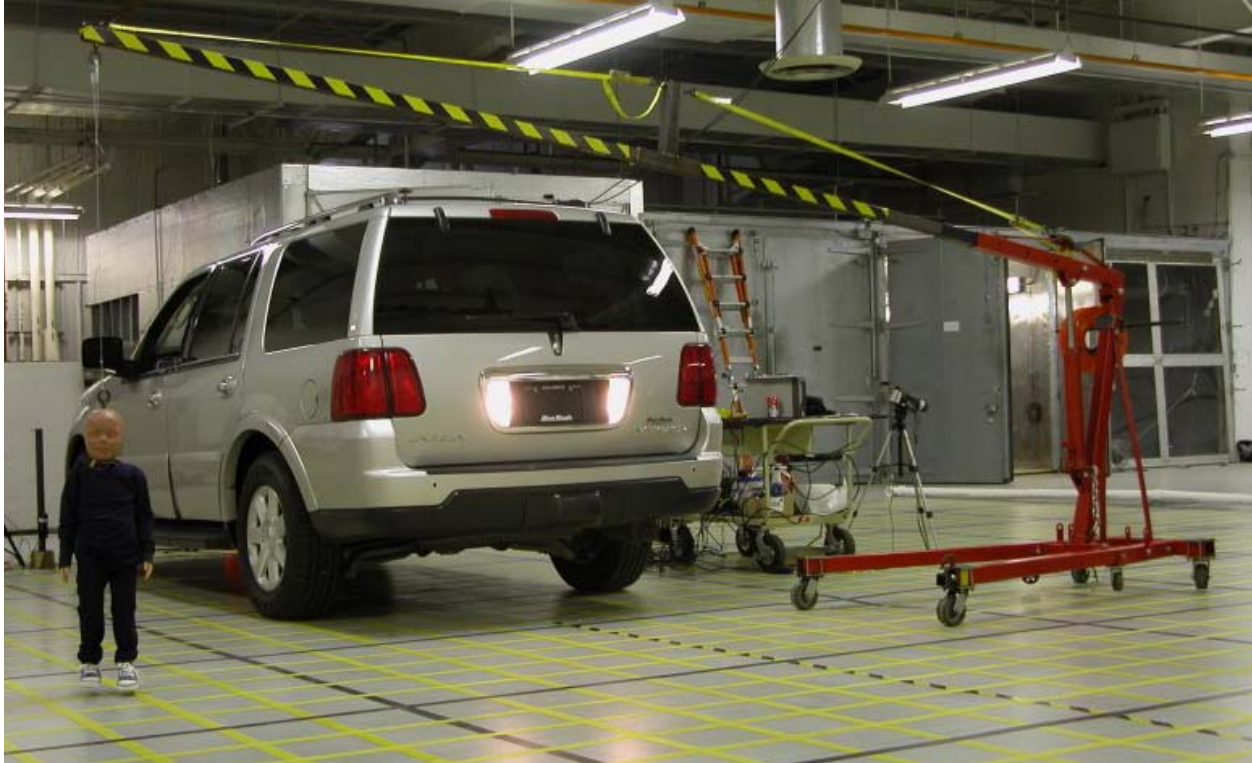
Figure 22. Hoist and Boom Apparatus with 3-year-old ATD on Indoor Field of View Measurement Grid
