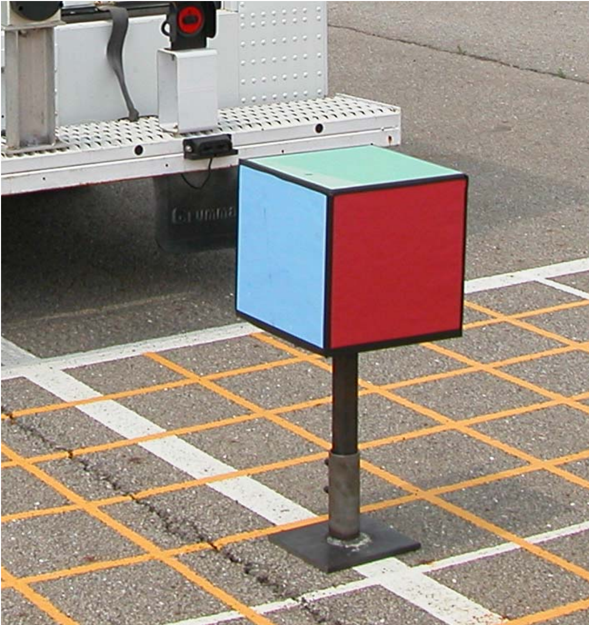
Figure 26. Cube Used for Image Distortion Determination
