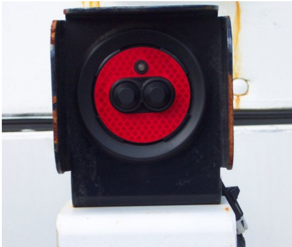
Figure 1. Eagle Eye Ultrasonic Sensor
