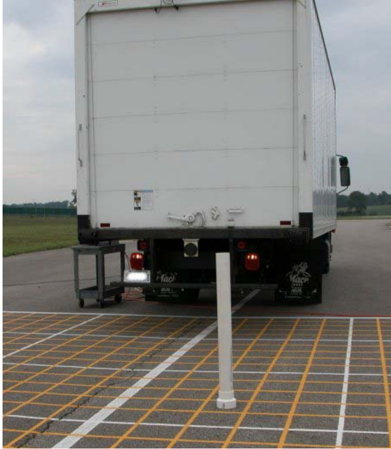
Figure 20. ISO 40-inch pole Set Up on Indoor Field of View Measurement Grid Behind a Light Vehicle
