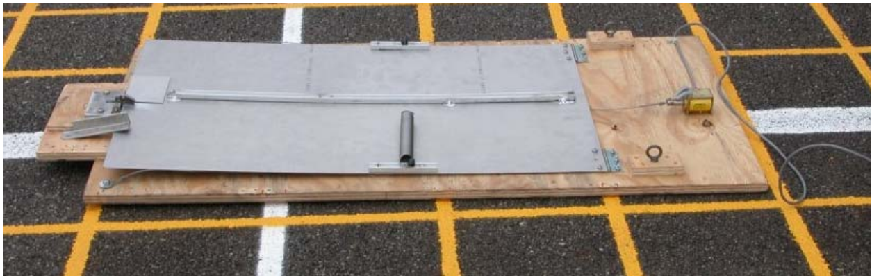
Figure 24. Response Time Fixture (Down Position)
