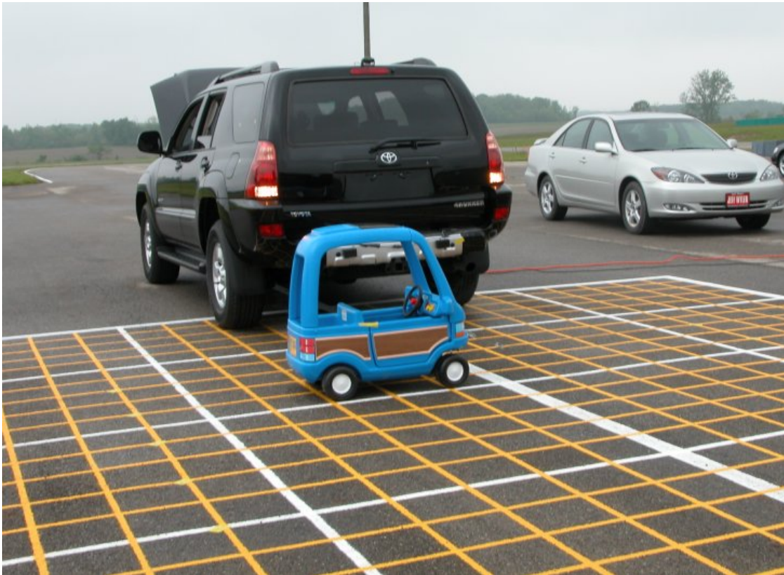
Figure 45. Photograph of Toy Car Outdoor Dynamic Test Trial
