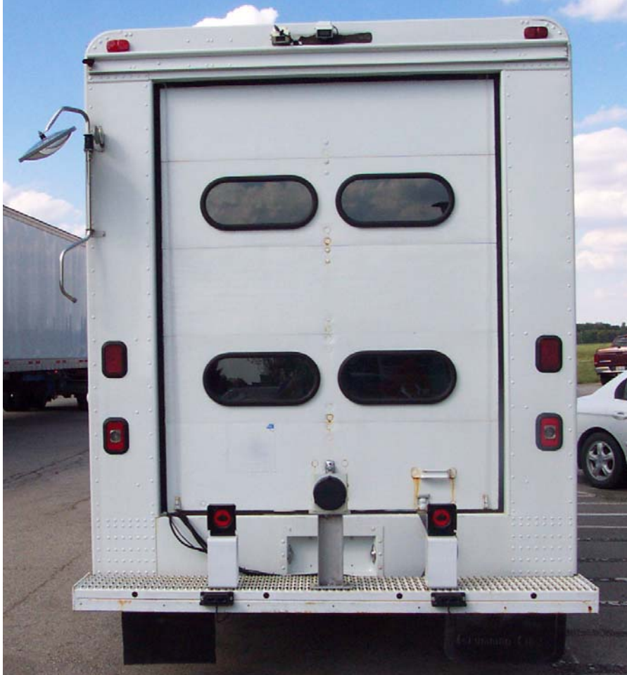
Figure 17. Rear of the 1996 Grumman-Olson 4x2 Step Van Showing Sensor Showing Installed Sensor, Camera, and Mirror Locations
