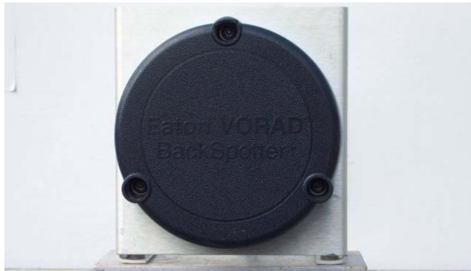
Figure 5. Vorad Backspotter Radar Sensor
