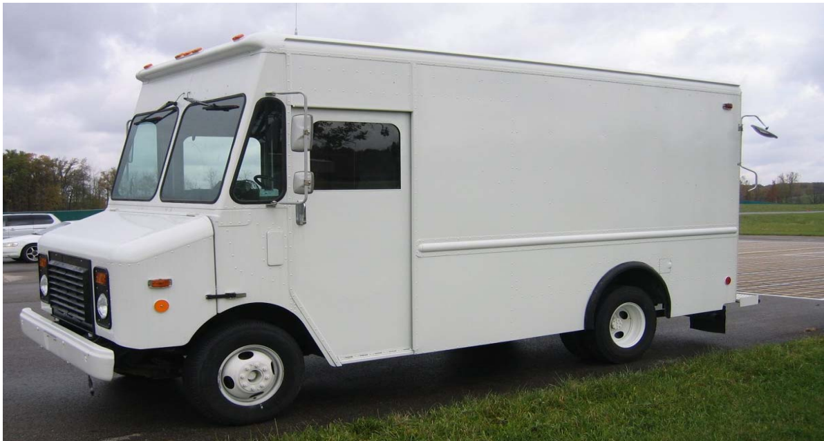
Figure 13. 1996 Grumman-Olson 4x2 Step Van Showing Flat Left Side-view Mirror and Rear Cross-view Mirror
