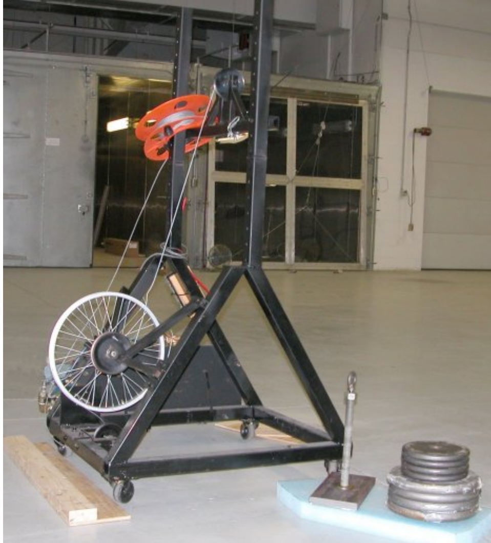
Figure 23. Pulley System Used for Controlled Speed Dynamic Tests
