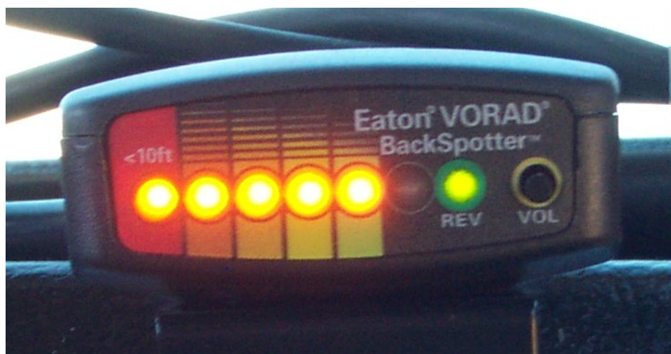
Figure 6. Vorad Backspotter Audio-visual Display
