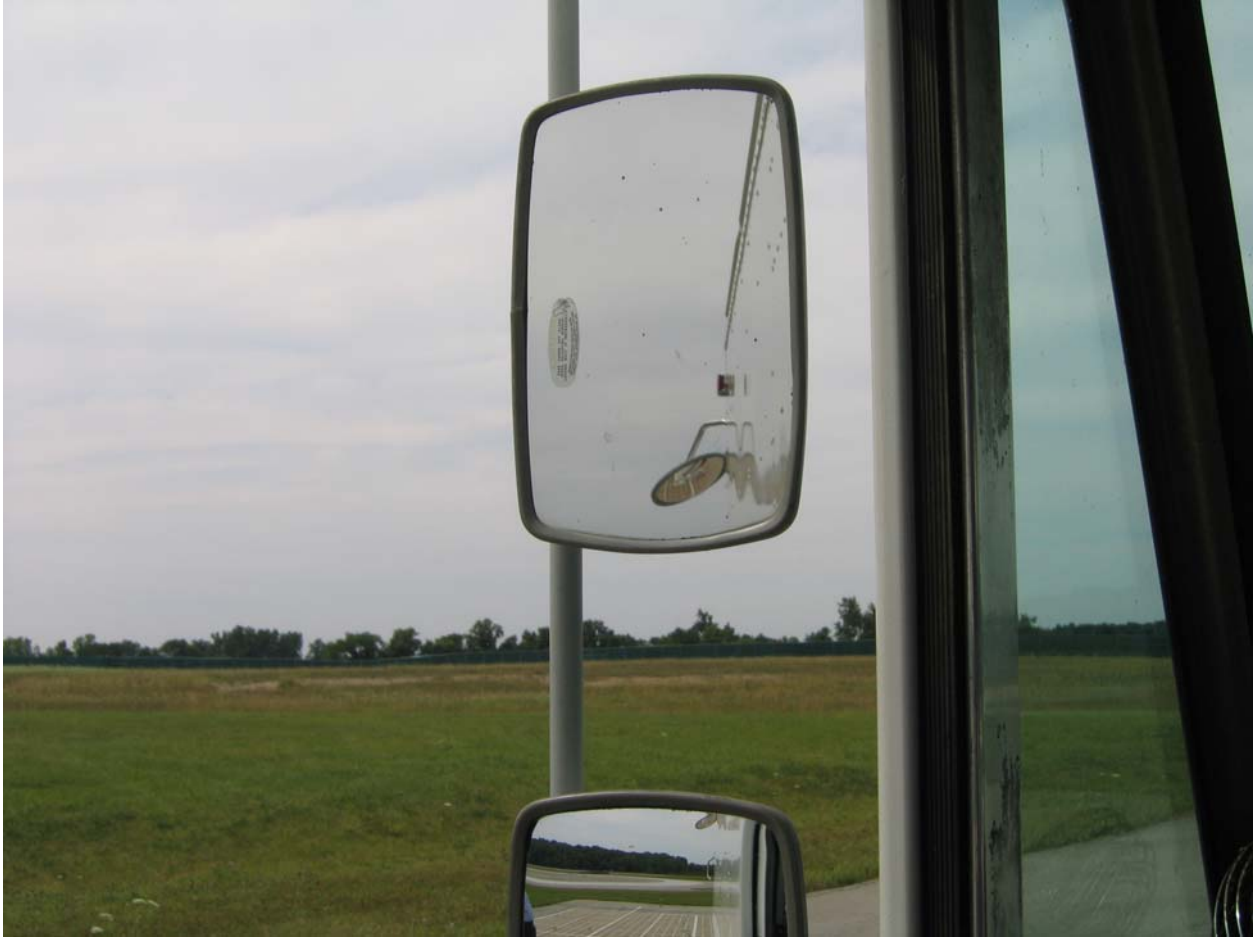
Figure 14. Driver's View of the Rear Cross-view Mirror as Seen in the Planar Side-view Mirror on the 1996 Grumman-Olson 4x2 Step Van
