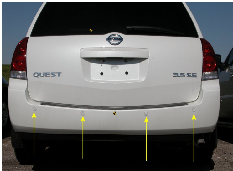
Figure 5. Nissan Quest sensor locations
