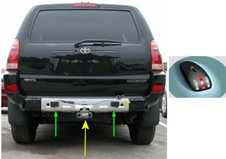
Figure 7. Guardian Alert sensors and visual display
