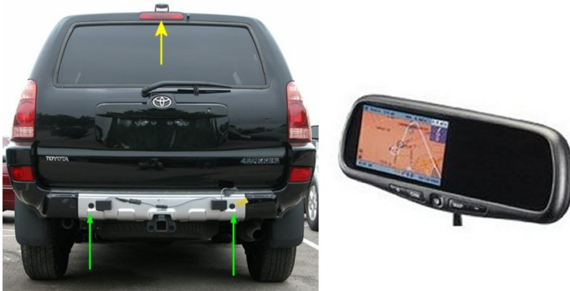
Figure 10. Audiovox system sensor and camera locations and rearview mirror video display
