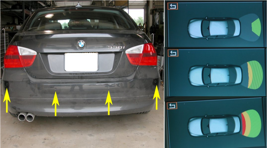
Figure 4. BMW 330i sensor locations and graphical display
