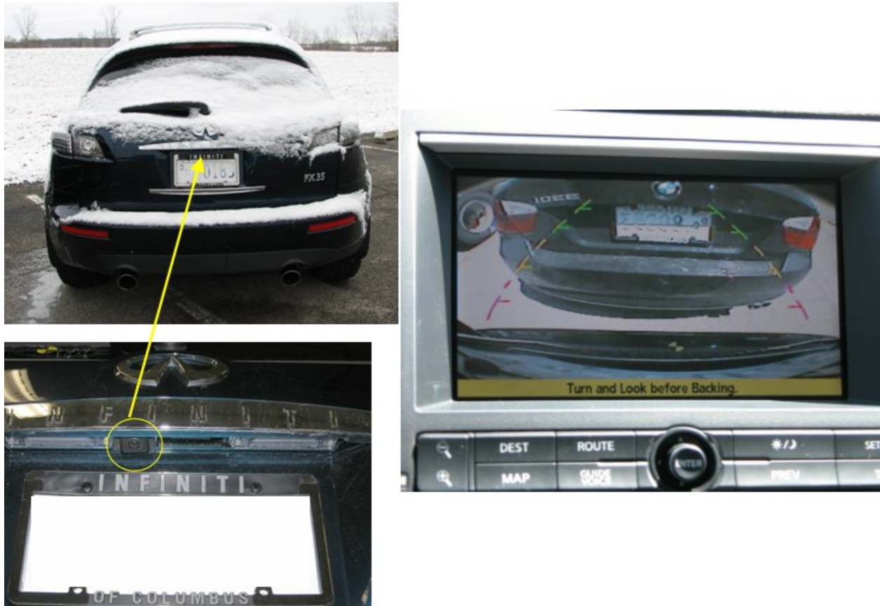
Figure 11. Infiniti FX35 camera location and video display
