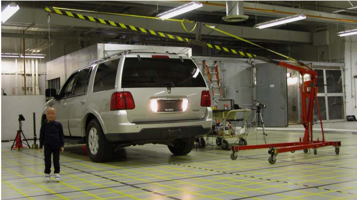
Figure 16. Hoist and boom apparatus with 3-year-old ATD on indoor test grid
