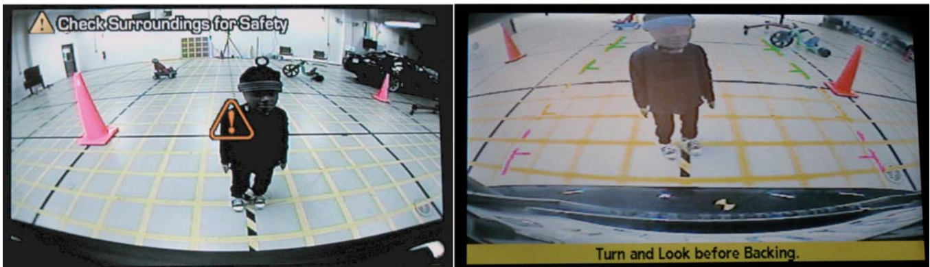
Figure 44. 3-year-old ATD at 2 feet from rear bumper as displayed by Cadillac Escalade (left) and Infiniti FX35 (right) rear video systems.
