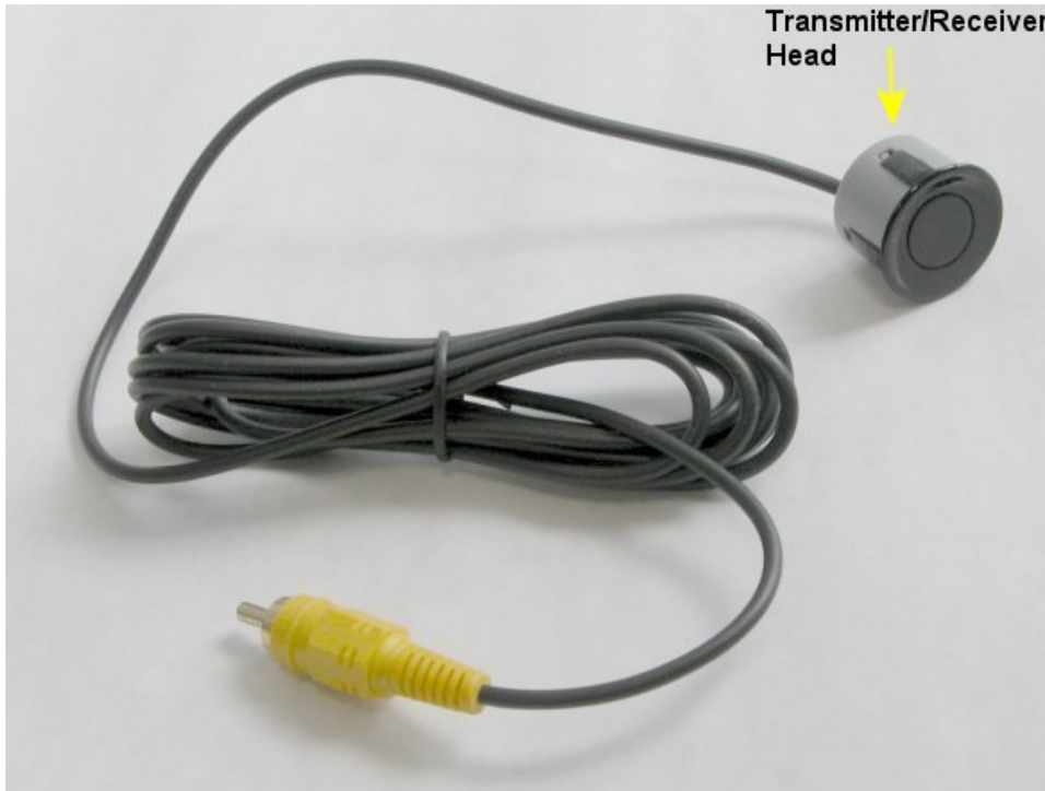
Figure 2. Example of an ultrasonic sensor
