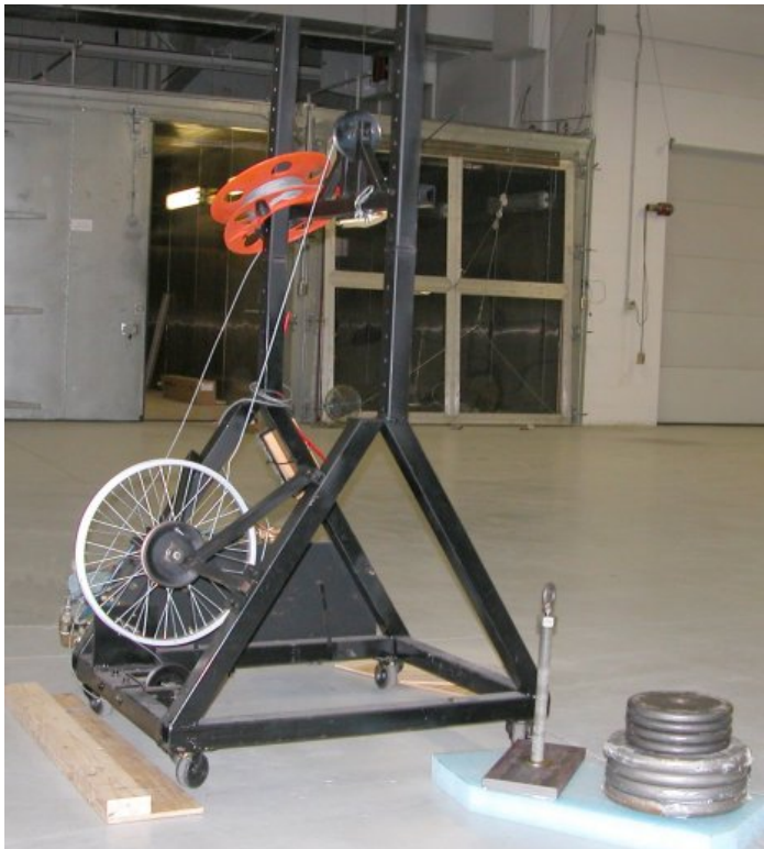
Figure 17. Pulley system used for controlled speed dynamic tests.
