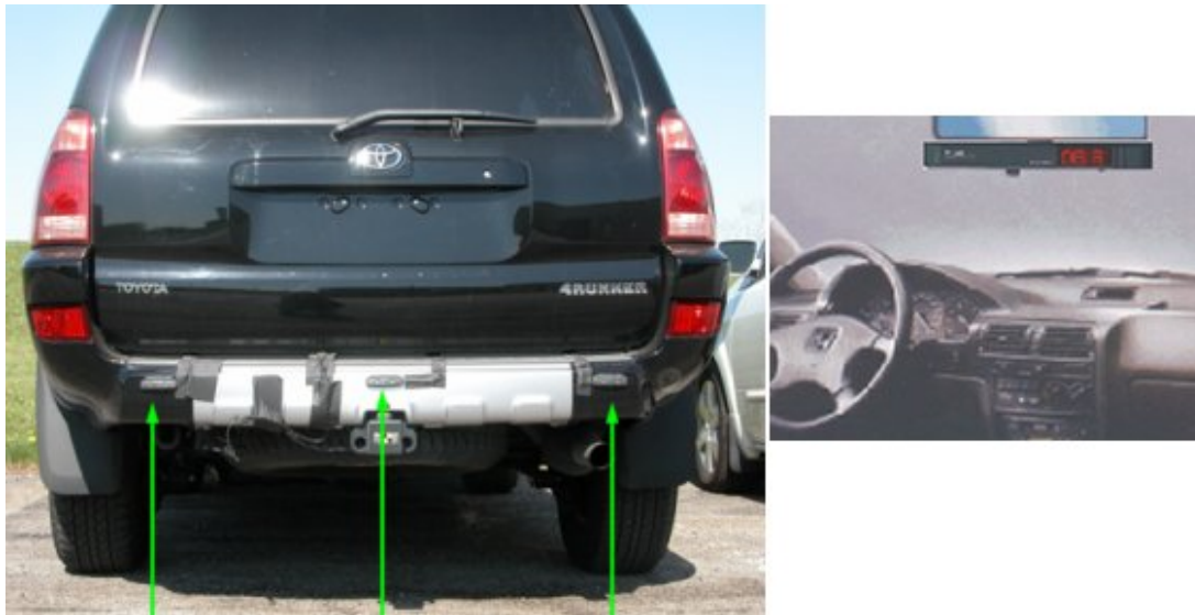
Figure 6. Poron sensors and LED distance visual display
