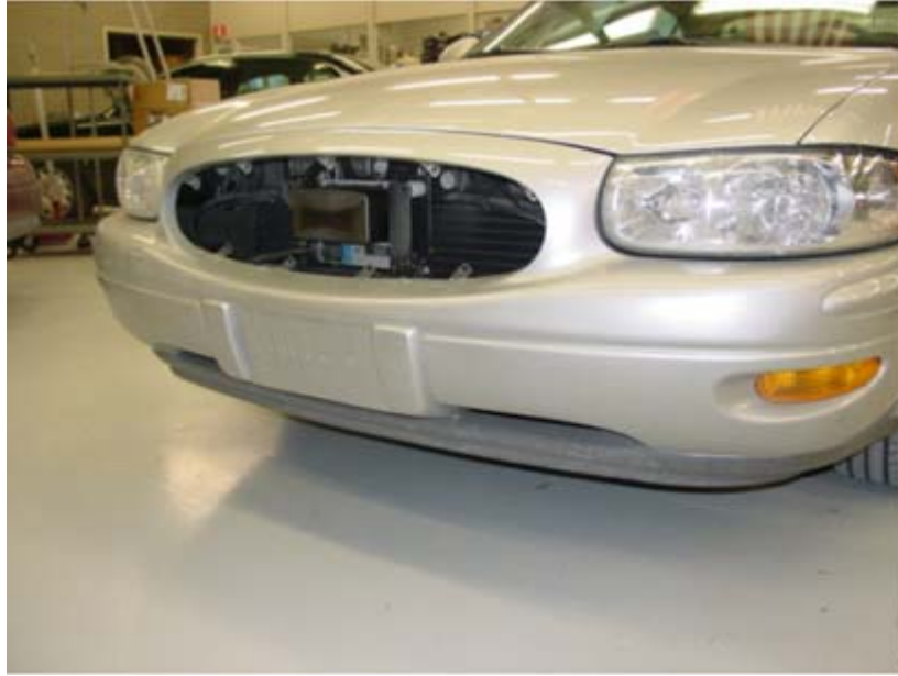
Figure 29: Radar with Front Grill Removed
