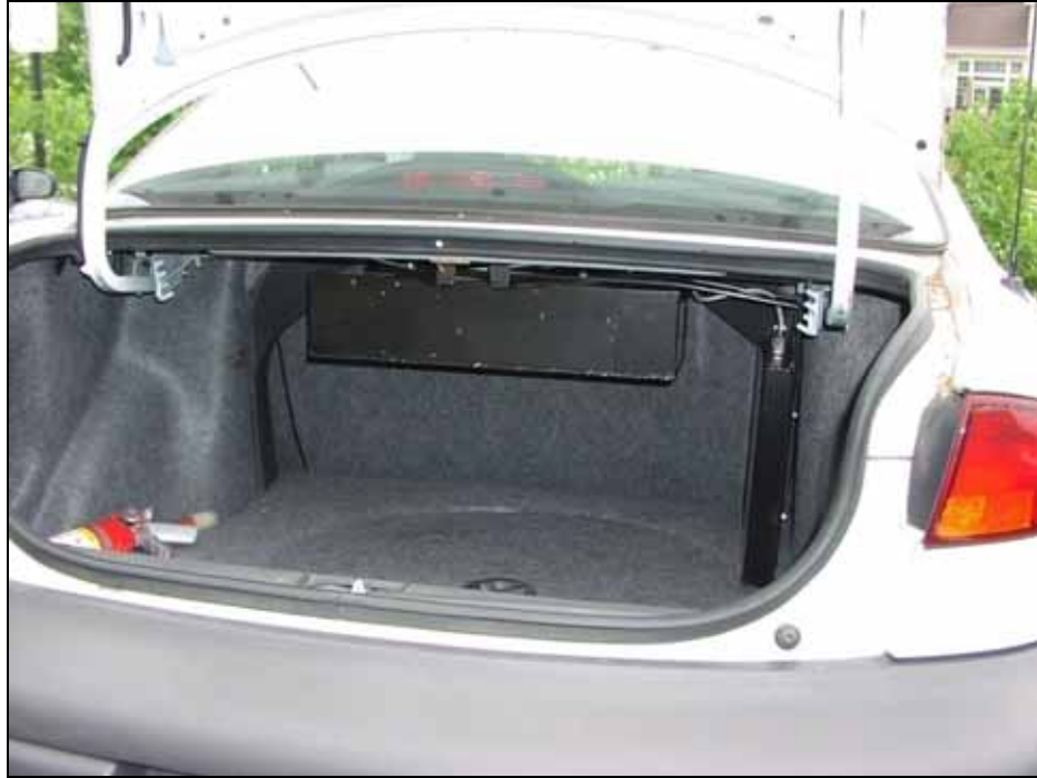
Figure 3. The Main DAS Unit Mounted Under the Package Shelf of the Trunk
