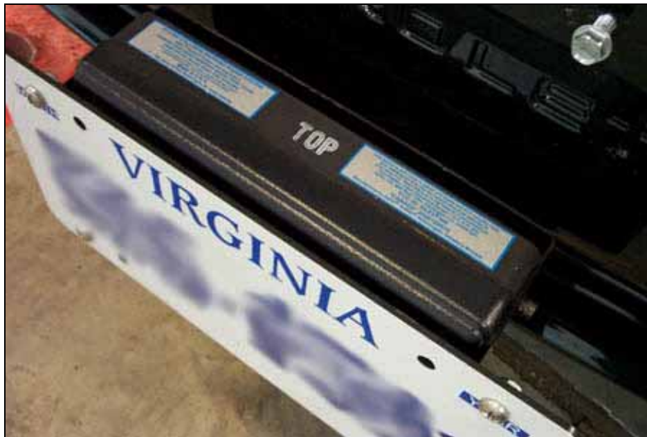
Figure 4. Doppler Radar Antenna Mounted on the Front of a Vehicle, Covered by a Mock-Up of One of the Plastic License Plates Used for This Study
