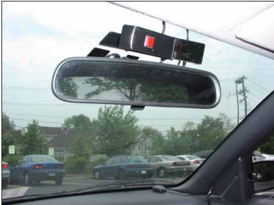
Figure 5. The Incident Pushbutton Box Mounted Above the Rearview Mirror.
