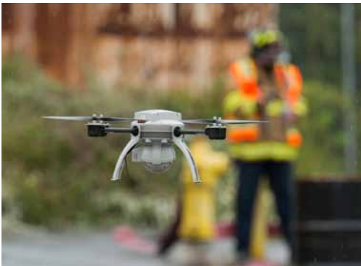
Alaska Test Range flight using an Aeryon Scout, at the Firefighters Training Facility, Fairbanks, Alaska (Jay Skaggs)
