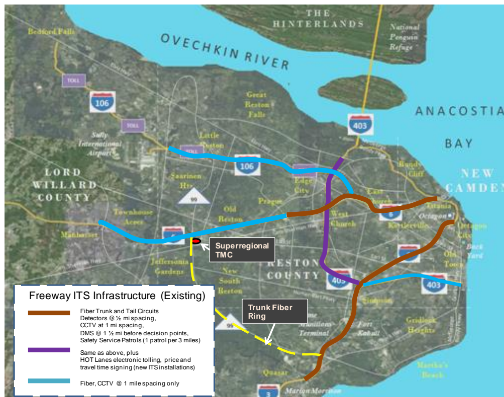
Figure 5-3: New Camden/Northern Jeffersonia Freeway ITS Infrastructure
