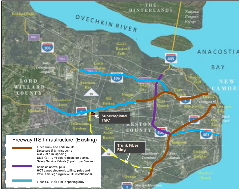
Figure 2-3: NCNJ Freeway ITS Infrastructure
