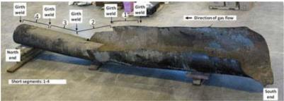
28-foot-long ruptured section of pipeline at laboratory facilities at the NTSB Training Center, Ashburn, VA (<u>Download full-sized version of image</u>)
