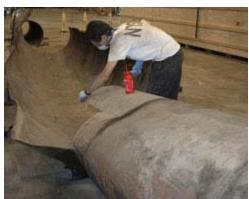
View of ruptured section of pipeline with investigator cleaning a fracture surface (<u>Download full-sized version</u>)
