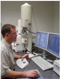
NTSB investigator using a scanning electron microscope to examine a pipeline fracture surface (<u>Download full-sized version</u>)
