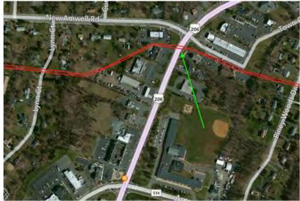
West Side of Rt 206. Excavation of Line 620. PSE&G Nat Gas Distribution pipeline crosses above BPL's line at an angle. Looking from west to east under Rt 206. 20" pipeline with 24" casing. Date 12/13/2012
