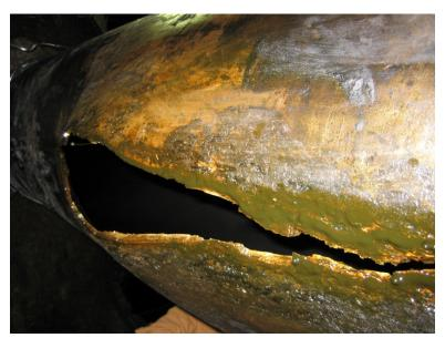
Photo 3: Failed "fish-mouth" section of pipe
