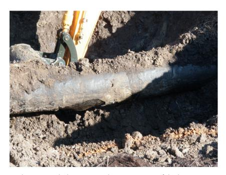
Photo 1: Failed Section with Opening at 6 o'clock position
