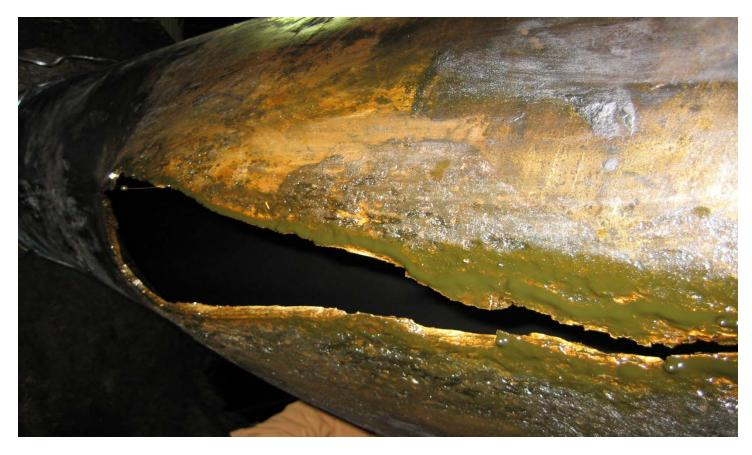
Shell Ho-Ho Pipeline Failed Pipeline Segment 11-19-2010 2:20PM
