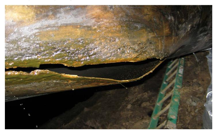
Shell Ho-Ho Pipeline Failed Pipeline Segment 11-19-2010 2:21PM
