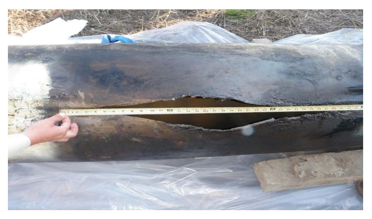
Shell Ho-Ho Pipeline Measurement of Ruptured Section 11-20-2010 3:49PM
