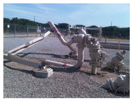
Failure of RV Support System. I-Beam is 90 degree from proper for maximum support. No 45 degree braces to counter moment applied by relief force.
