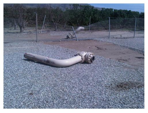
Two (2) Relief vents thrown clear after failure of relief support system.
