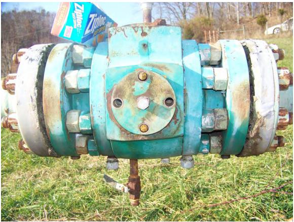
Photo 7 Columbia Gas Transmission Ripley Storage valve failure Manufacturer Tulsa Valve ANSI 900 4 inch Photo by ED Clarkson West Virginia Gas Pipeline Safety
