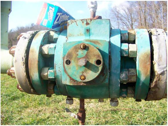
Photo 9 Columbia Gas Transmission Ripley Storage valve failure Manufacturer Tulsa Valve ANSI 900 4 inch Photo by ED Clarkson West Virginia Gas Pipeline Safety
