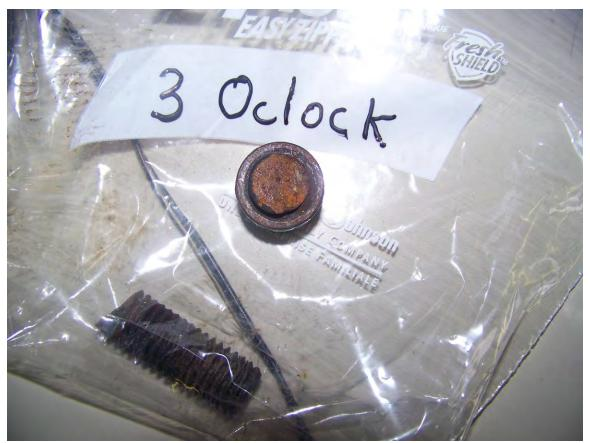
Photo 4 Columbia Gas Transmission Ripley Storage valve failure Manufacturer Tulsa Valve ANSI 900 4 inch Trunnion cover bolt Photo by ED Clarkson West Virginia Gas Pipeline Safety
