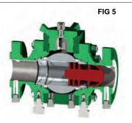
To Launch the pig open [Counterclockwise] the valve and the pig will be launched downstream.
