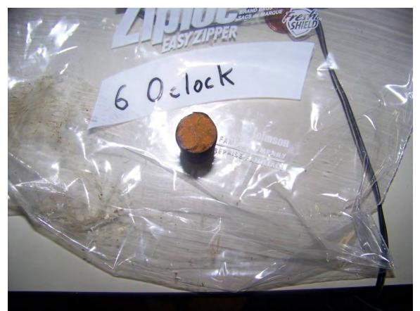
Photo 2 Columbia Gas Transmission Ripley Storage valve failure Manufacturer Tulsa Valve ANSI 900 4 inch Trunnion cover bolt Photo by ED Clarkson West Virginia Gas Pipeline Safety
