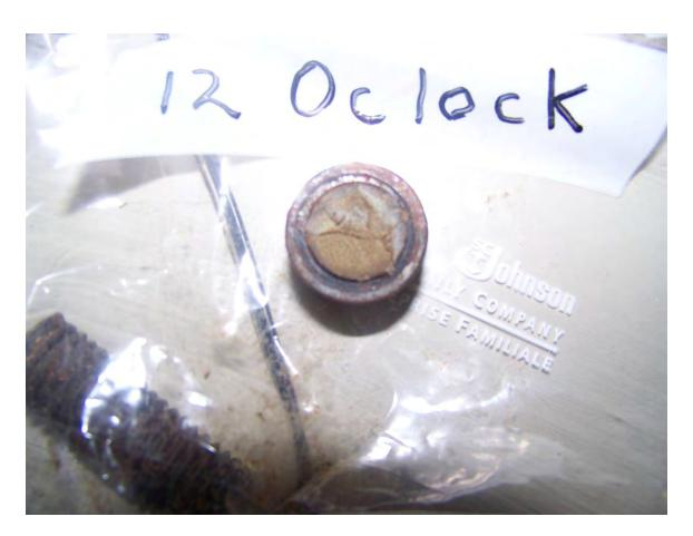
Photo 5 Columbia Gas Transmission Ripley Storage valve failure Manufacturer Tulsa Valve ANSI 900 4 inch Trunnion cover cap Photo by ED Clarkson West Virginia Gas Pipeline Safety
