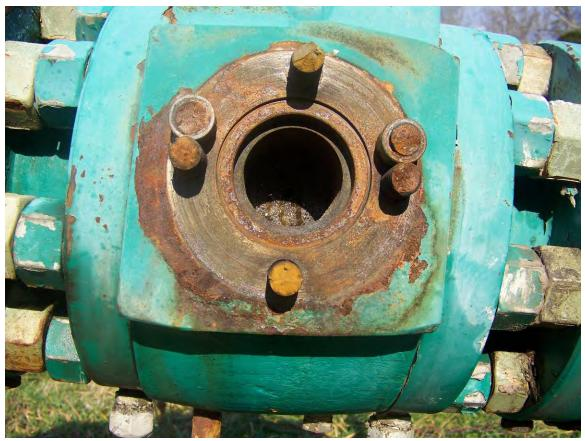
Photo 1 Columbia Gas Transmission Ripley Storage valve failure Manufacturer Tulsa Valve ANSI 900 4 inch Shut- off pigging valve X-59-W7308 Photo by ED Clarkson West Virginia Gas Pipeline Safety
