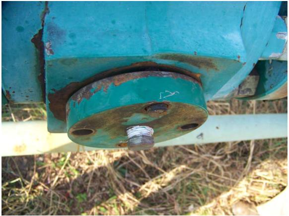
Photo 6 Columbia Gas Transmission Ripley Storage valve failure Manufacturer Tulsa Valve ANSI 900 4 inch Photo by ED Clarkson West Virginia Gas Pipeline Safety
