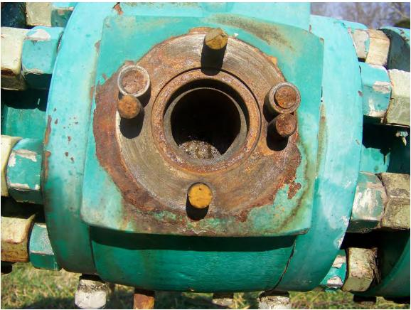
Photo 12 Columbia Gas Transmission Ripley Storage valve failure Manufacturer Tulsa Valve ANSI 900 4 inch Photo by ED Clarkson West Virginia Gas Pipeline Safety
