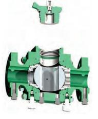
Remove the Pig. Caution: Valve is under pressure use caution when removing pigs. Flush the valve clean.
