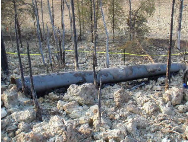
Figure 9. Low Energy Failure pipe section
