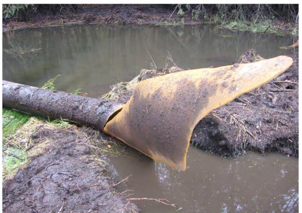
Figure 5: End of severed 37.1 foot section of pipeline
