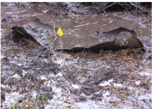
Figure 3: Severed 9 foot section of pipeline
