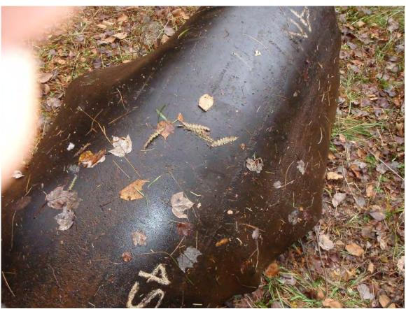
Figure 9: Piece 4 exhibiting corrosion
