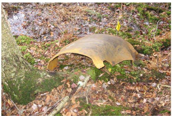
Figure 4: Severed 4.7 foot section of pipeline, piece 4
