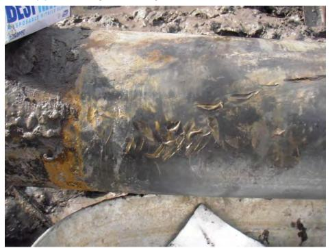
Additional photo showing mechanical damage
