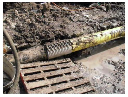
Closer view of coating damage
