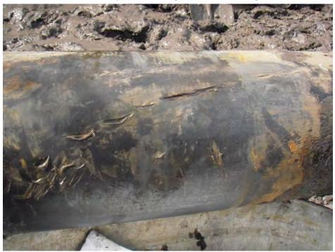
CFPL cut out 13-feet of the jet fuel pipeline that included the damaged section and sent it to Exponent Failure Analysis Associates for metallurgical and mechanical testing.
