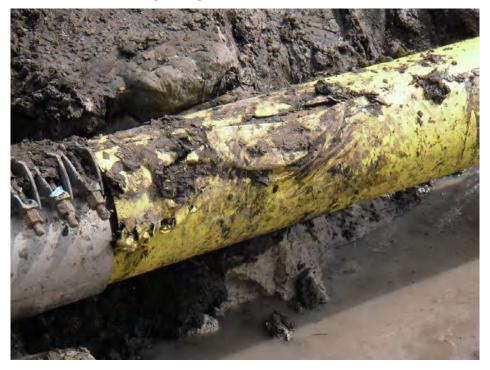
The mechanical damage was evident after leak clamp removal. The pipe leaked from one of the gouges shown in the photograph.
