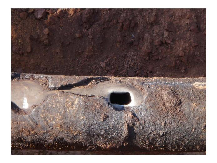
Photo taken facing north, showing additional damages to pipeline from excavation prior to puncture
