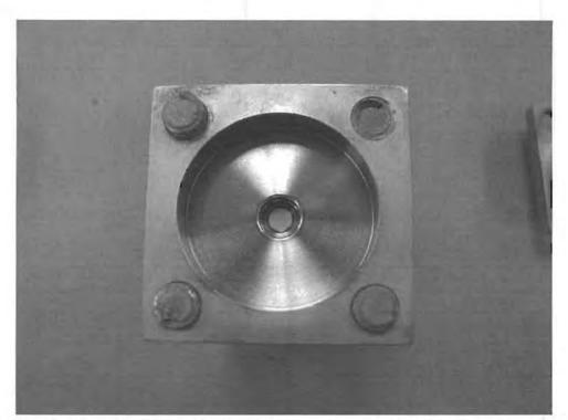
**Photo 4:** A closer view of the fracture faces on the screws. Screw # 1 is the upper left, screw # 2 is at the upper right, screw # 3 is at the lower right and screw # 4 is at the lower left in the photograph.
