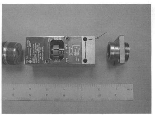
Photo 2: A closer view of the failure location. One of the failed screws is just visible in this view and is marked with the arrow.
