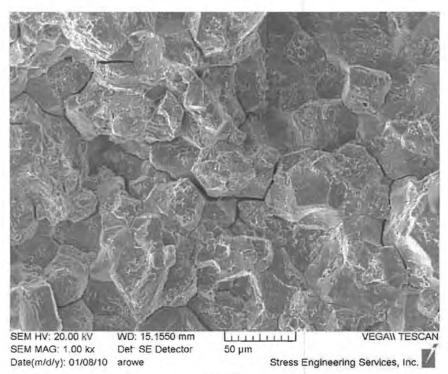
Photo 7: The fracture surface on screw #1 following ultrasonic cleaning. The fracture face appears typical of hydrogen stress cracking.
