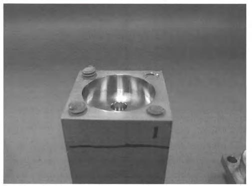
Photo 3: A view of the outer ends of all the failed screws.
