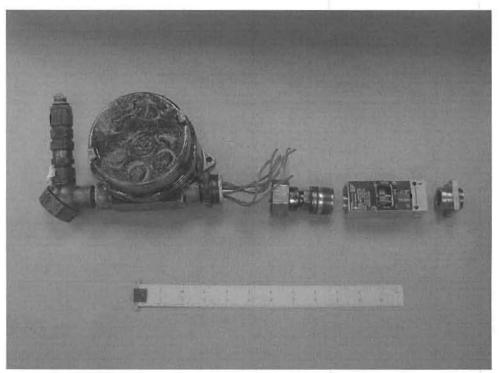
**Photo 1:** The failed switch supplied for this investigation. The failure occurred at the right end of the switch, as shown in this photograph.
