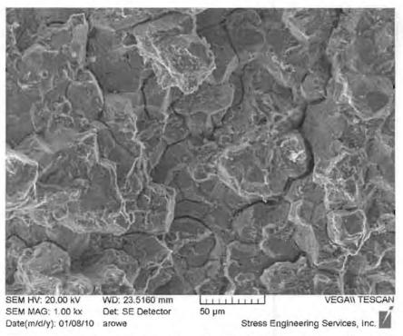
**Photo 8:** The fracture surface found on screw # 3. The structure is essentially identical to that shown in Photograph 7.
