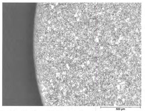
Photo 6: A view of the microstructure in screw # 3. The structures in both screws are essentially identical and appear typical of a quenched and tempered high alloy steel.
