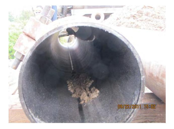
**Photo #2: Damage to the internal surface of the pipe (cut out).**
