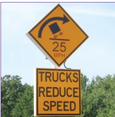
Figure 2: LEDs are embedded in the symbols and lettering on this truck warning sign.
