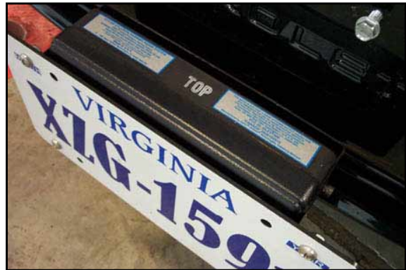
Figure 3. Doppler radar antenna mounted on the front of a vehicle, covered by one of the plastic license plates used for this study.
