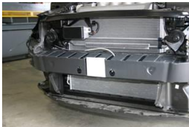
Figure 12: Front Radar Installation
