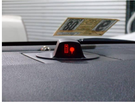
Figure 3 The Visual Display is Located on the Dash of the Experimental Vehicle
