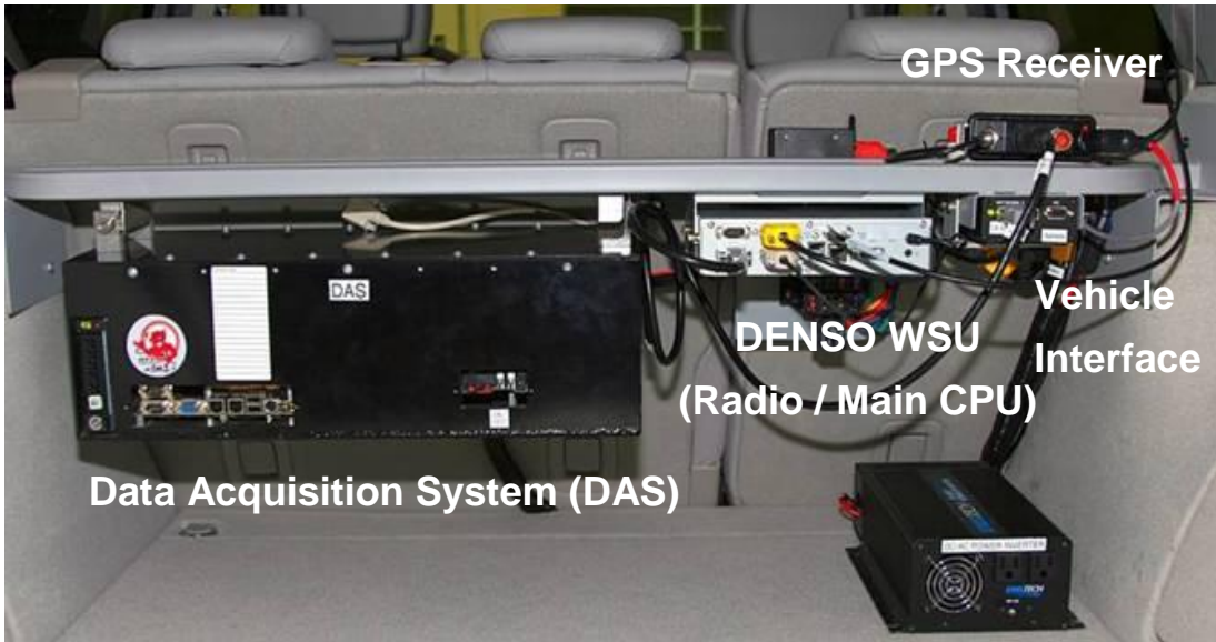
Figure 10: CICAS-V Components in the Vehicle
