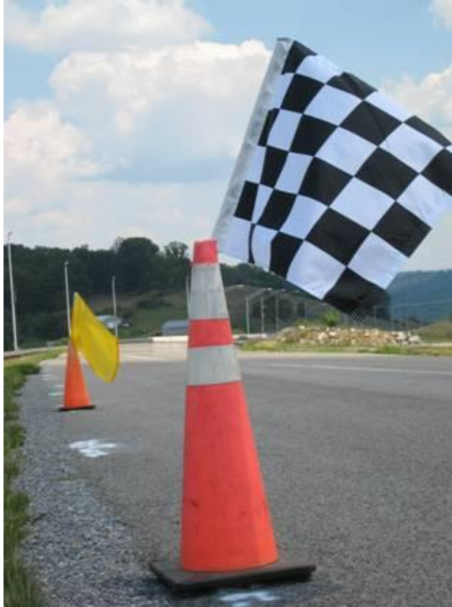
Figure 19: Cones with Flags Demarking the Warning Zone
