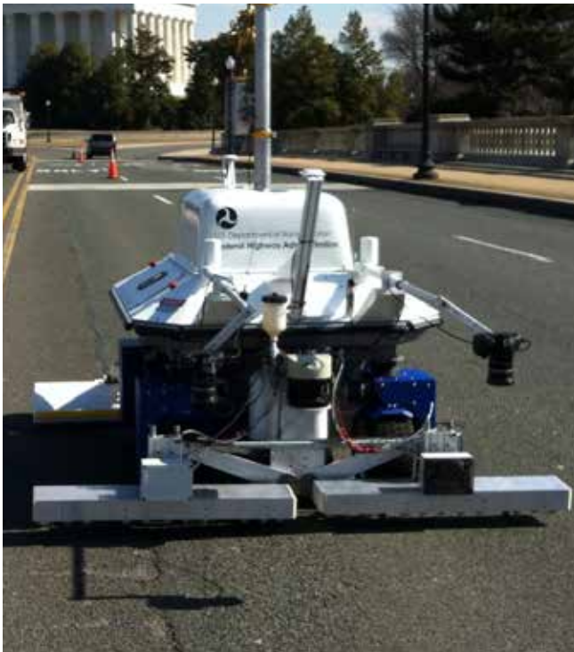
The RABIT™ bridge deck assessment tool is eight times faster than conventional methods at collecting data on the conditions of a bridge's deck and subsurface. (Image source: FHWA)
