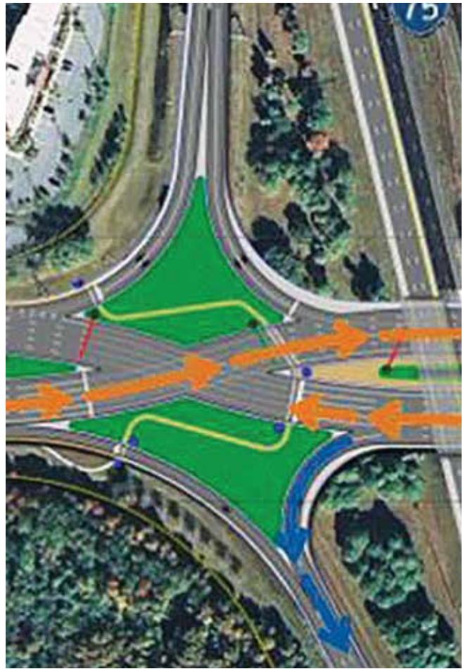
Diverging diamond interchanges reduce pedestrian conflicts at busy intersections near freeway ramps. (Source: Missouri DOT)
