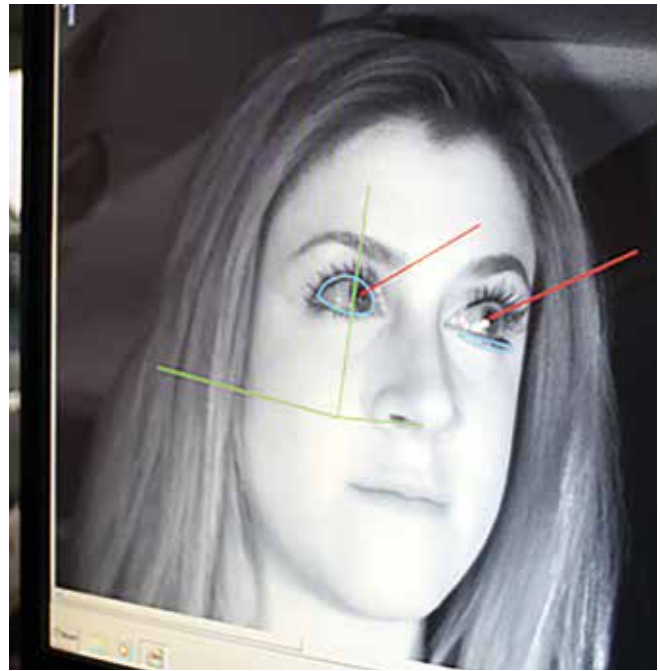
FHWA's field research vehicle can study drivers' eye movements in real world settings, collecting valuable data on driver distractions. (Image source: FHWA)
