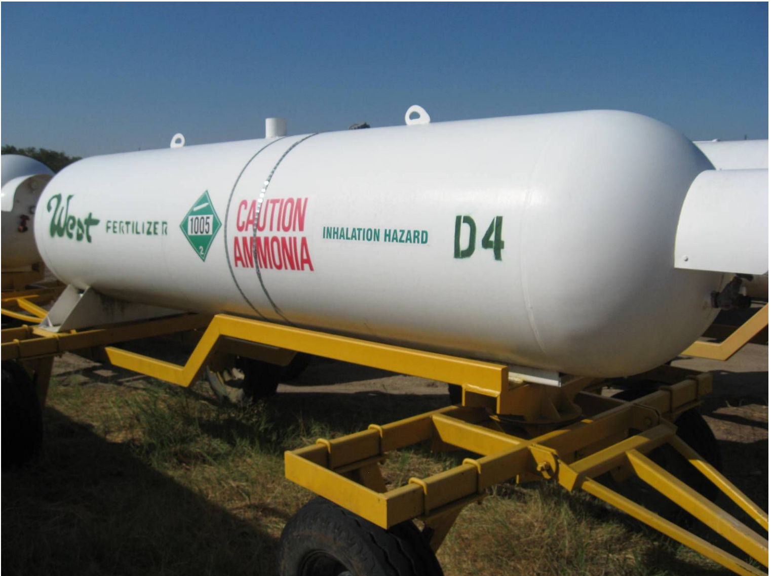
#D4 with required side placard & markings
