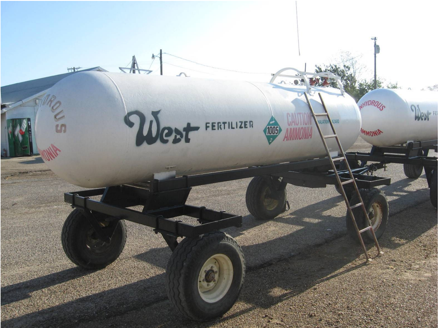
#G34 with required side placard & markings
