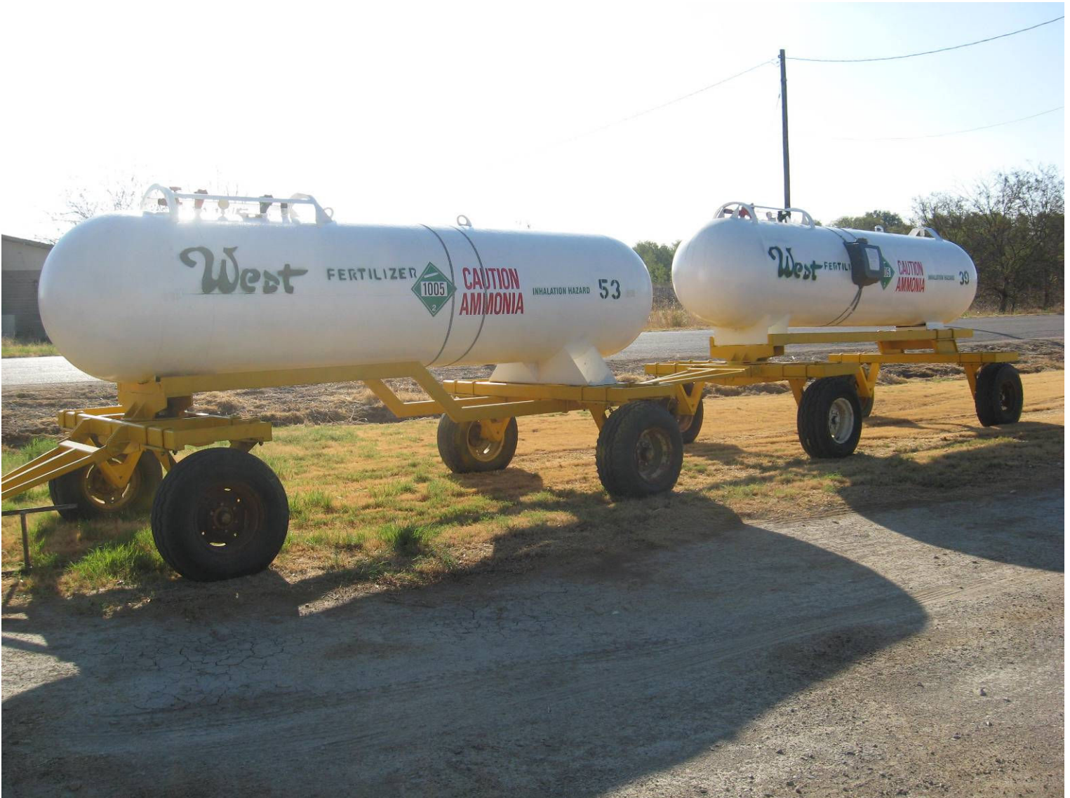
#53 & #39 with required side placards & markings; and missing front Non-Flammable Gas placards and 1005 & NH3 markings
