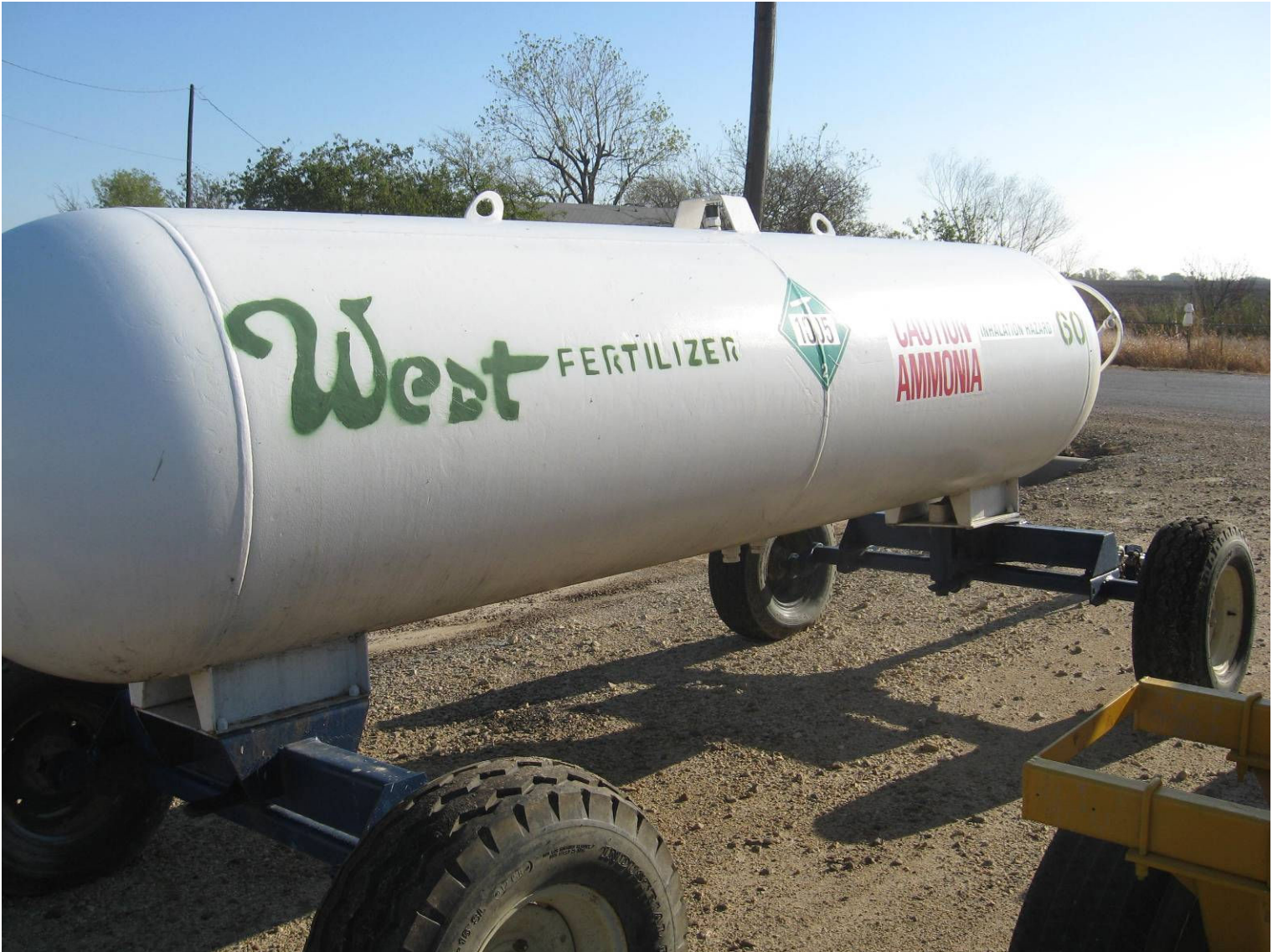
#60 with required side placards & markings
