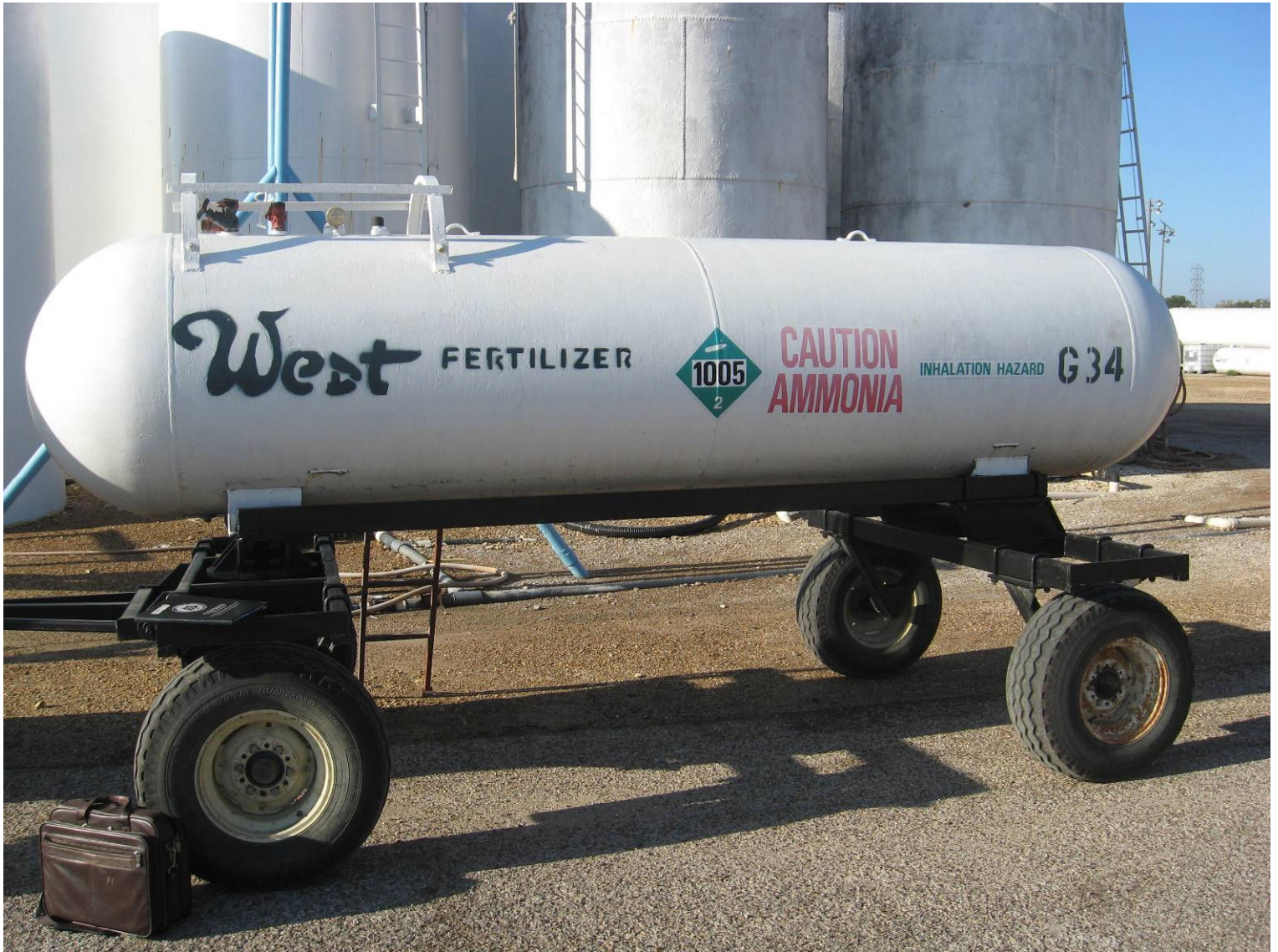
#G34 with required side placard & markings
