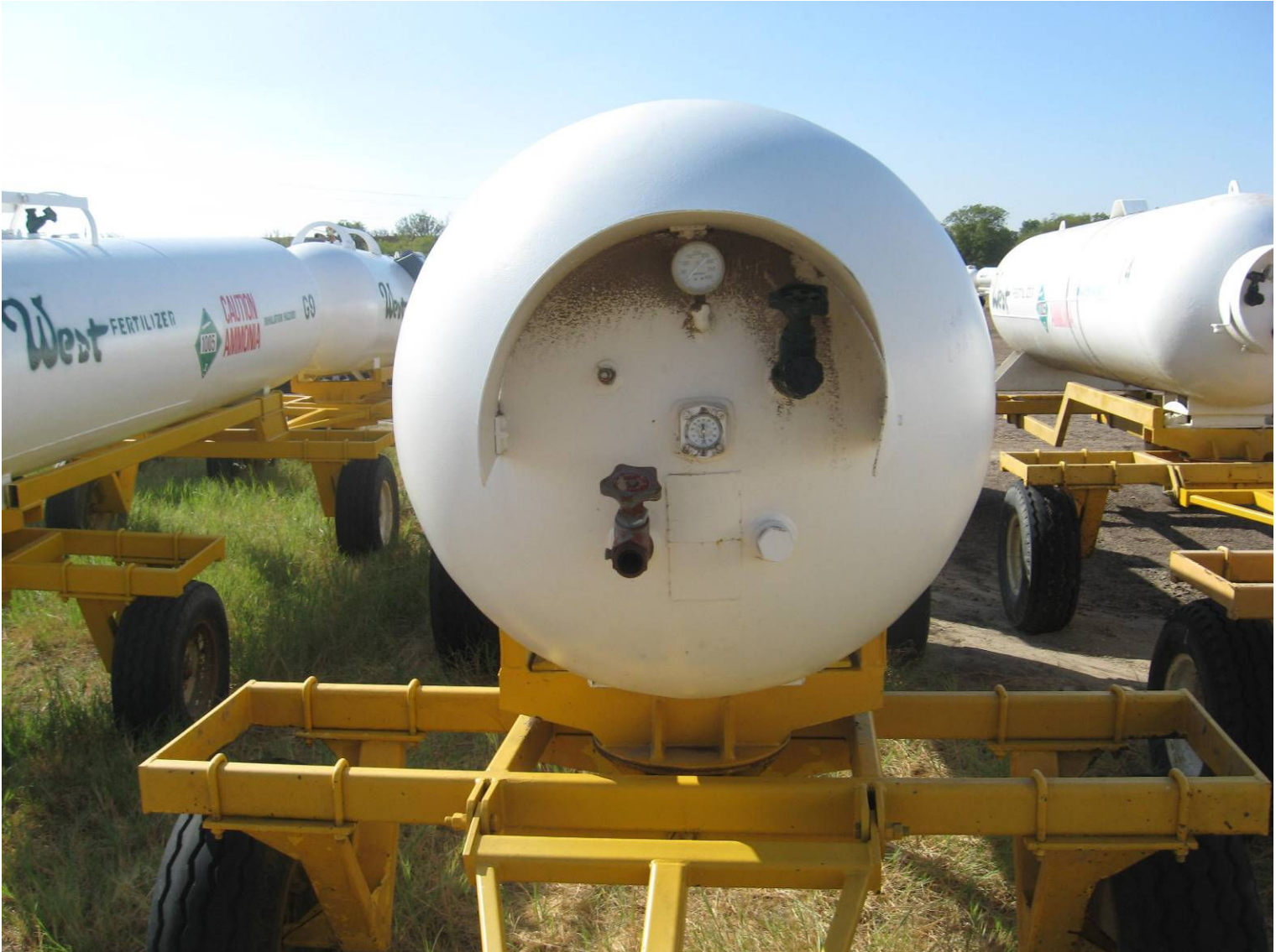
#D4 with illegible ASME data plate
