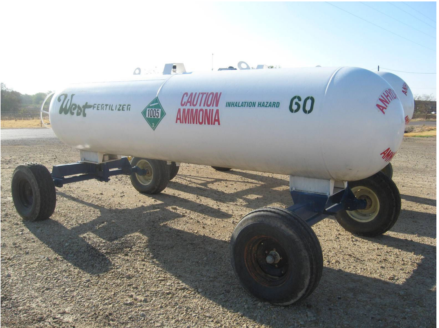
#60 with required side placards & markings
