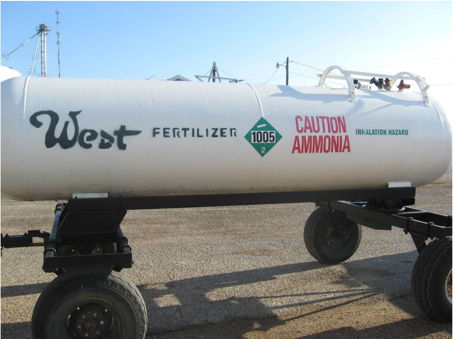
#71 with required side placard and markings
