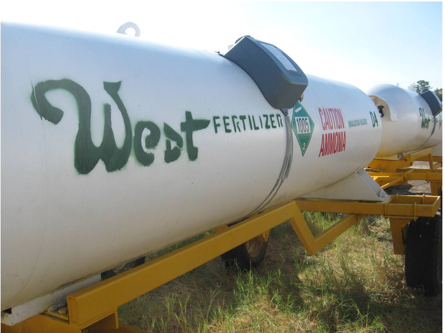
#D4 with required placard & markings
