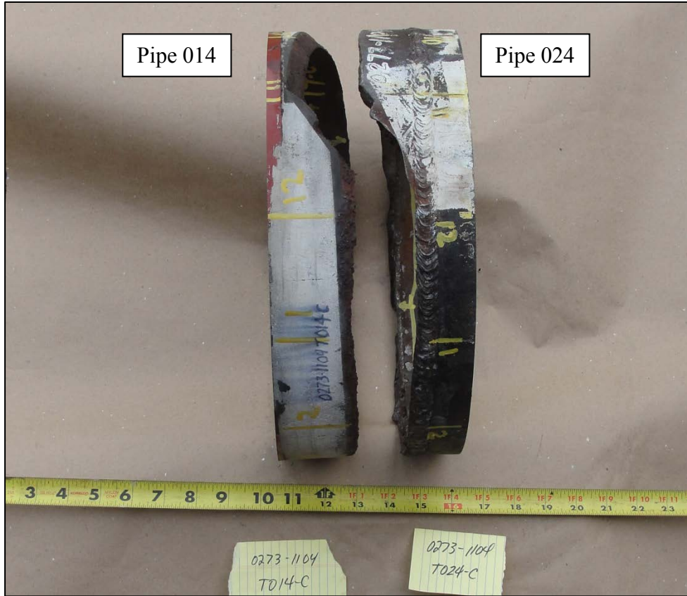
Figure 19. Pipe rings containing fracture surfaces
