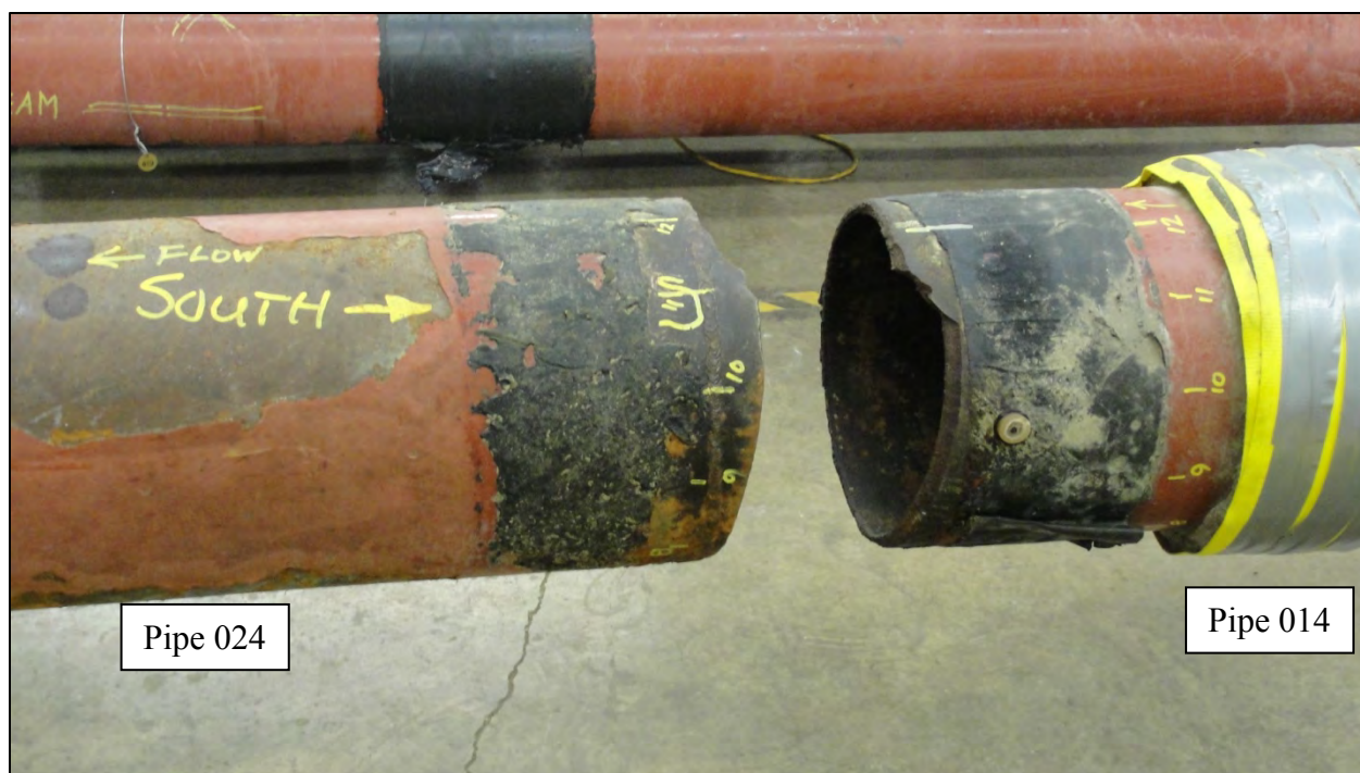
Figure 14. Fractured ends of the pipe aligned
