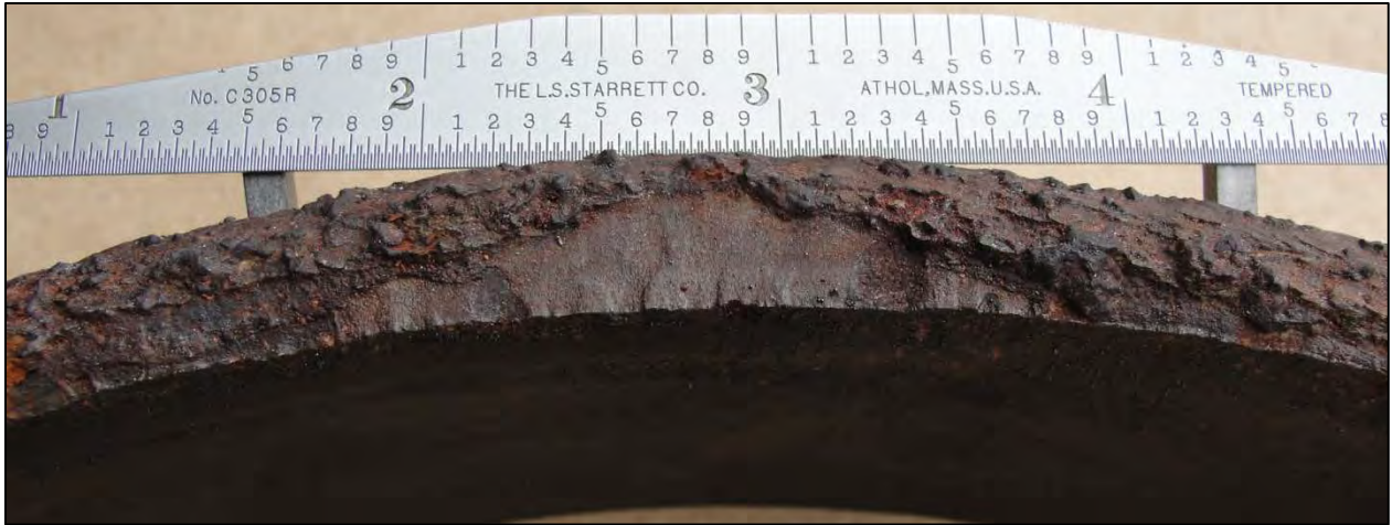
Figure 22. Fracture surface of Pipe 014 showing Feature “S”
