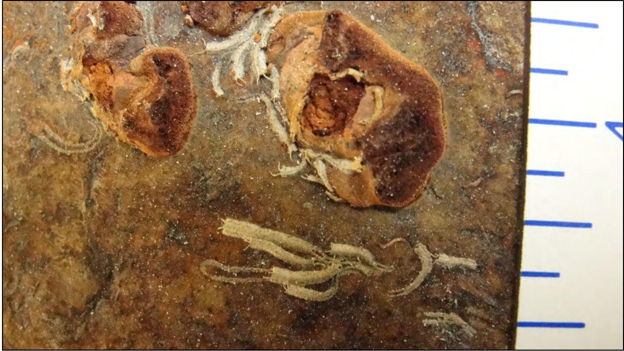
Figure 8. Detail of organisms on pipe surface
