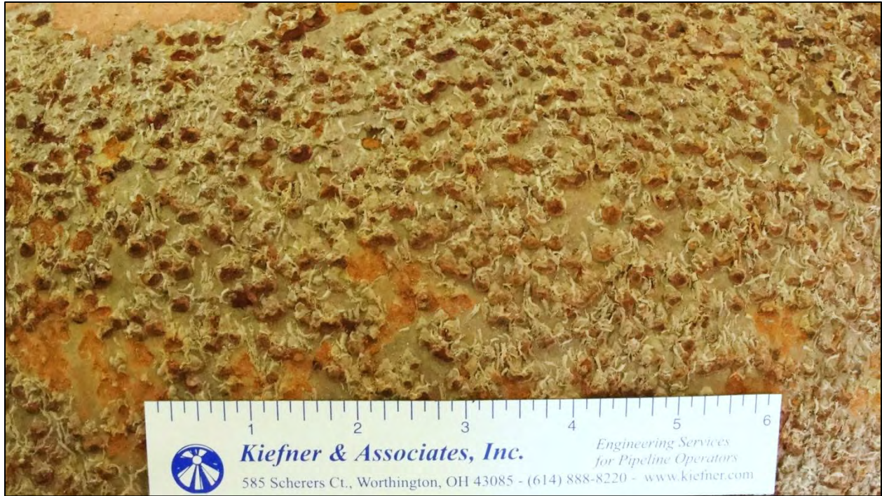
Figure 6. Organisms on Surface of Pipe 024
