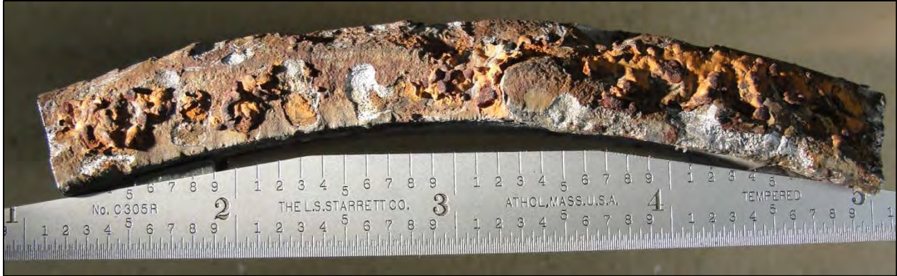
Figure 27. Fracture surface after cleaning with naphtha and Alconox (T014-C-2)
