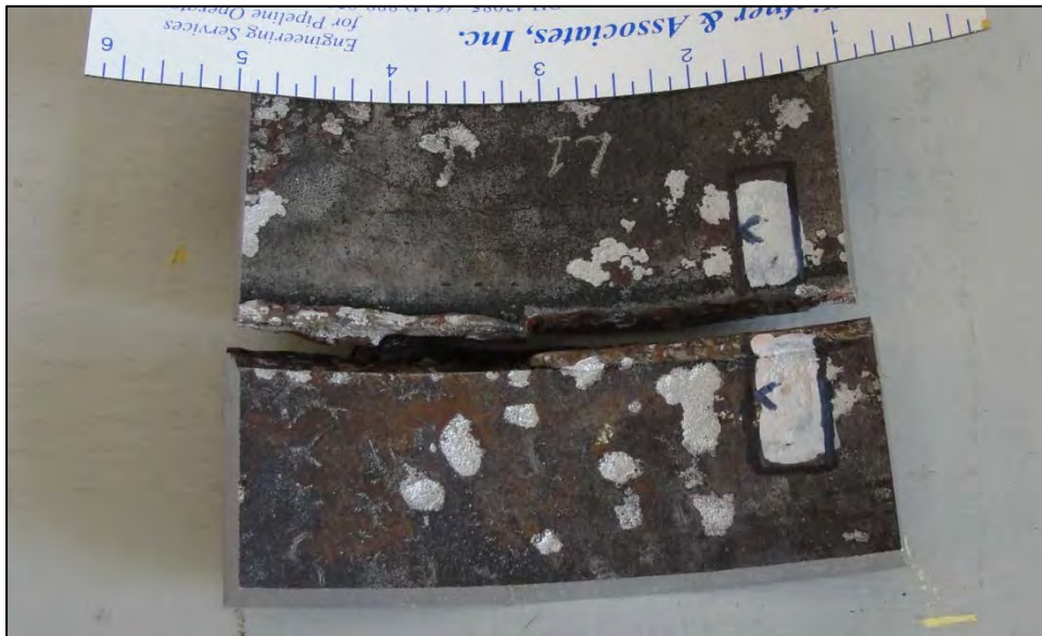
Figure 45. Location of metallographic sections through feature L
