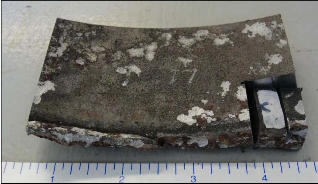
Figure 46. Location of metallographic section through feature L (T014-C-2)
