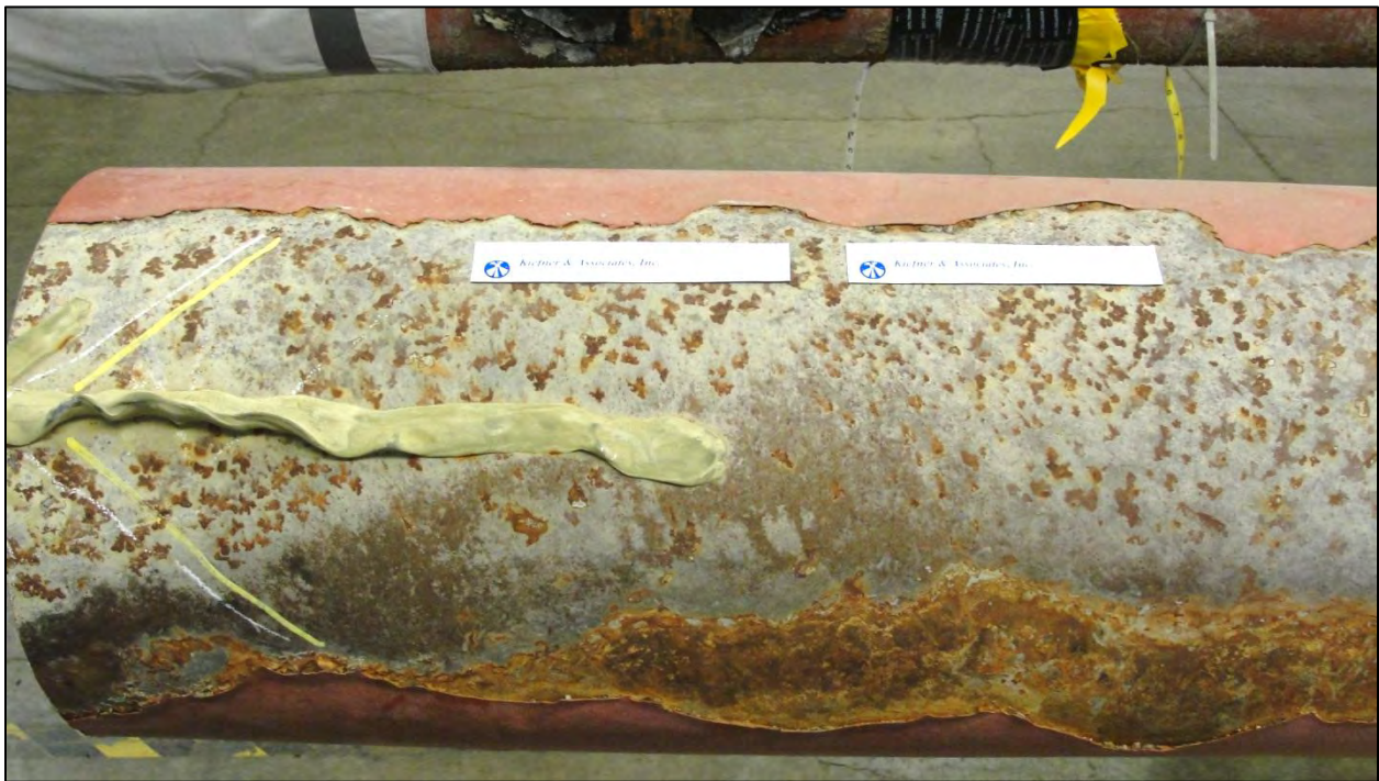
Figure 4. Area of coating erosion on Pipe 024
