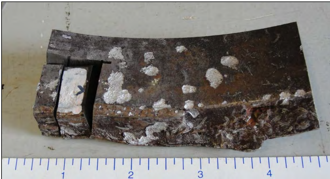
Figure 47. Location of metallographic section through feature L (T024-C-2)
