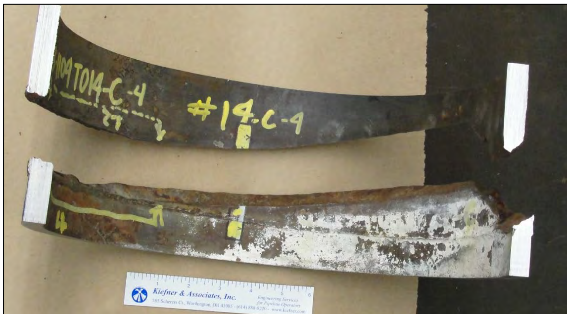
Figure 49. Location of metallographic section through shear portion of fracture
