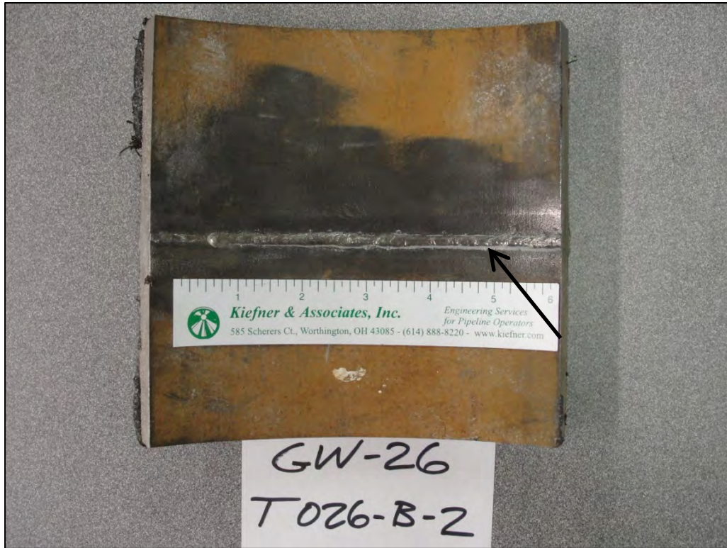
Figure 59. Internal surface of Coupon T026-B-2 showing MT indication
