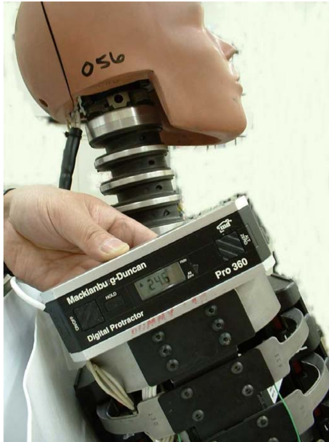
Figure 60. Adjusting the SID-IIsD in the fore/aft plane for pelvis certification tests
