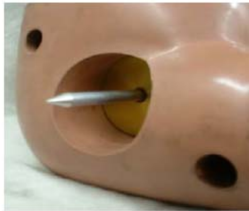
Figure 3. Threaded cylindrical tool installed at acetabulum
