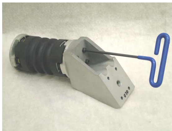
Figure 14. Removal of the neck from neck bracket
