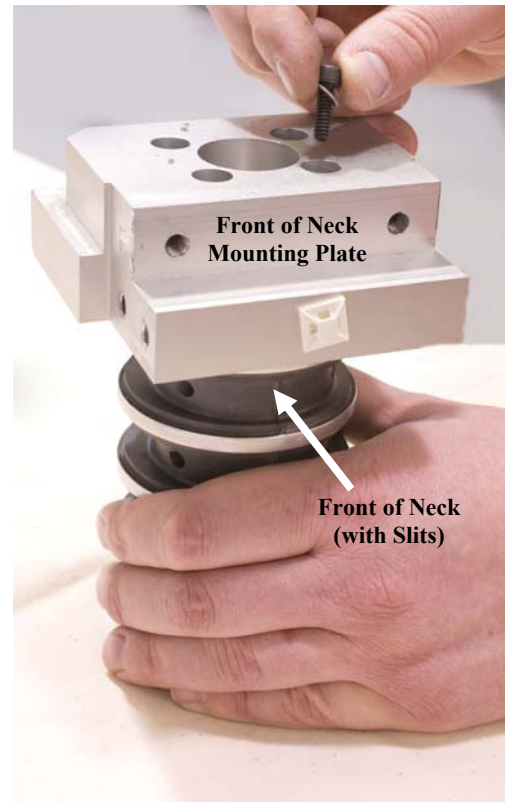
Figure 19. Assemble molded neck to neck mounting plate
