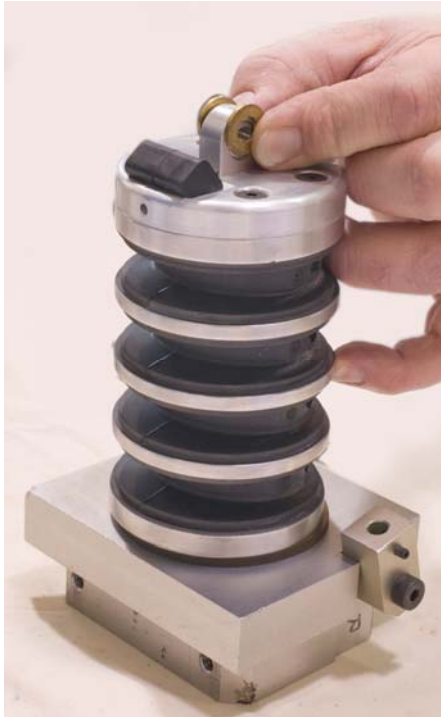
Figure 24. Install brass nodding joint washers
