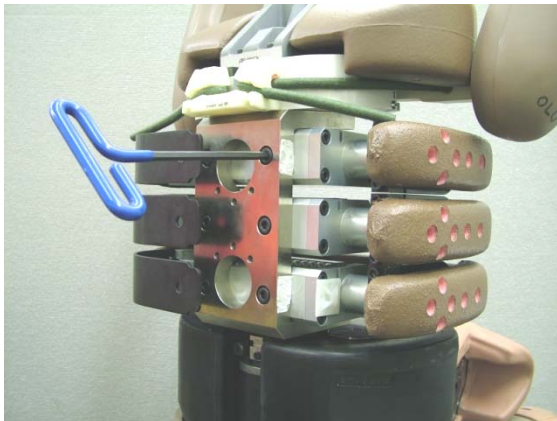
Figure 22. Removal of rib module
