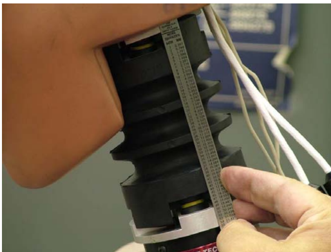
Figure 2. Checking for a straight neck before measuring sitting height
