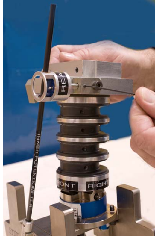
Figure 33. Tighten set screws for inner potentiometer pivot bracket
