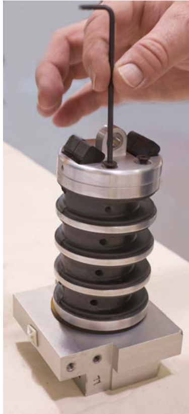
Figure 22. Reinstall neck nodding joint assembly
