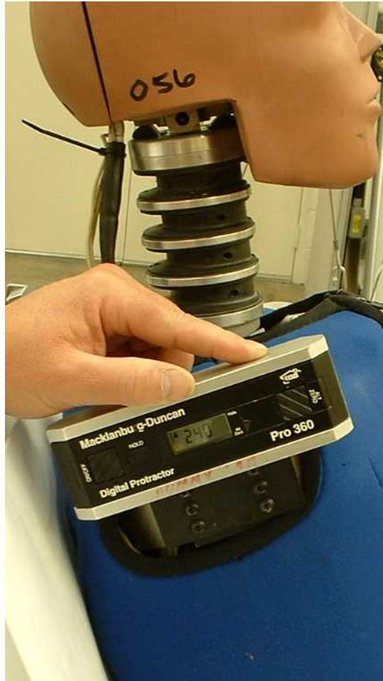
Figure 46. Adjusting the SID-IIsD in the fore/aft plane
