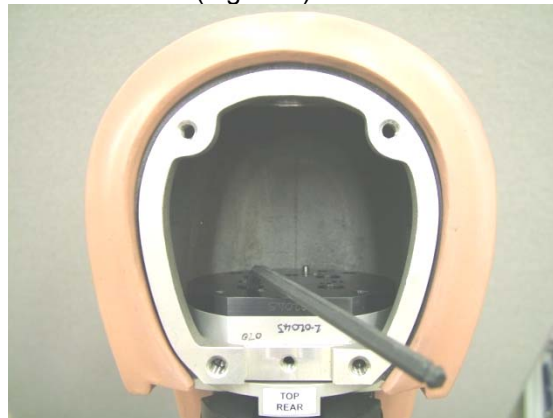
Figure 6. Removal of head from neck
