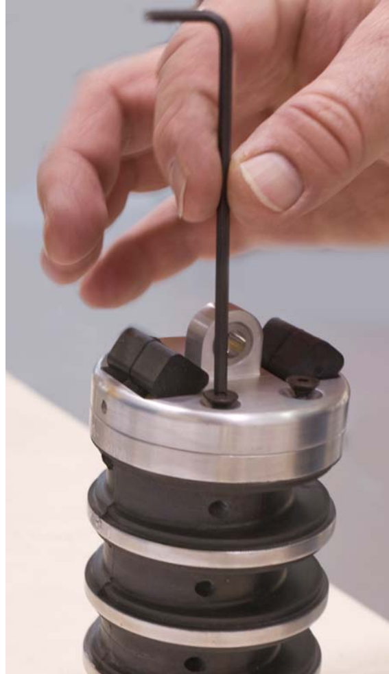
Figure 17. Removing the nodding joint assembly
