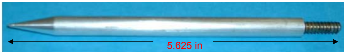
Figure 2. Threaded cylindrical tool
