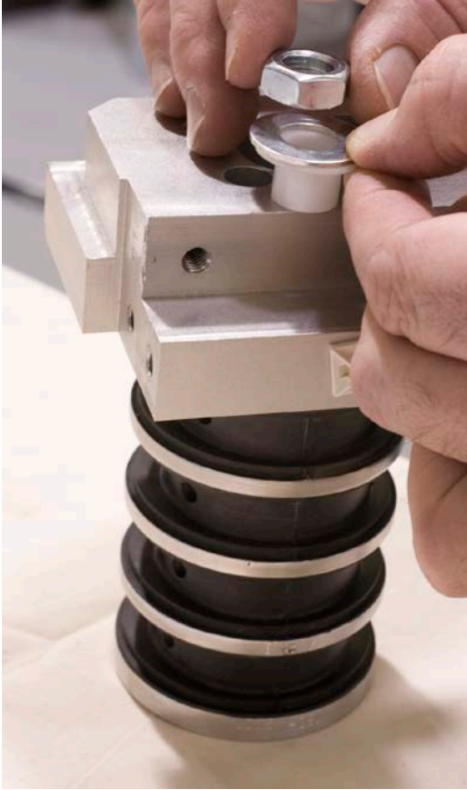
Figure 20. Install lower neck bushing, washer, and hex nut onto neck cable
