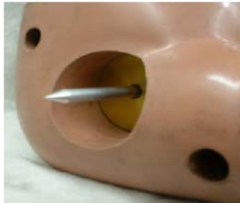
Figure 3. Threaded cylindrical tool installed at acetabulum
