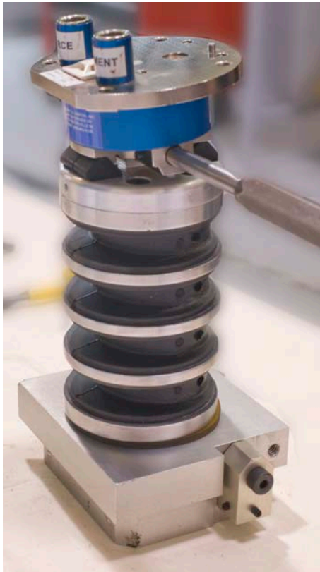
Figure 26. Align brass nodding joint washers with holes
