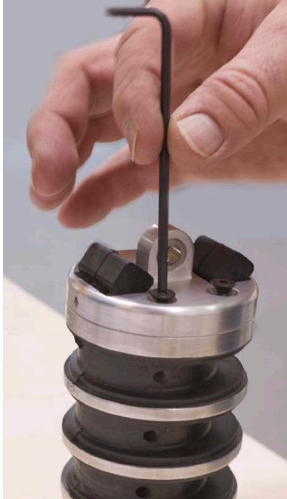
Figure 17. Removing the nodding joint assembly
