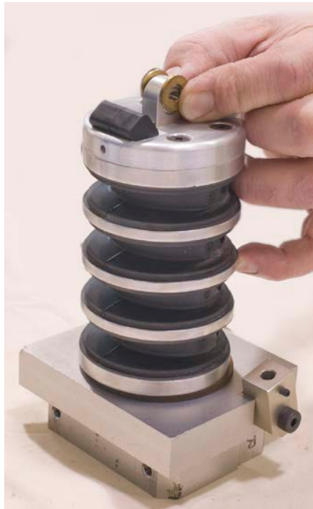
Figure 24. Install brass nodding joint washers
