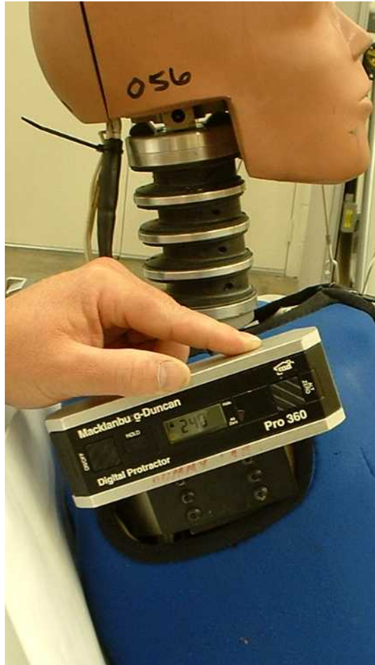
Figure 46. Adjusting the SID-IIsD in the fore/aft plane
