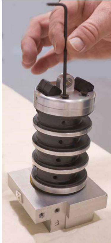
Figure 22. Reinstall neck nodding joint assembly
