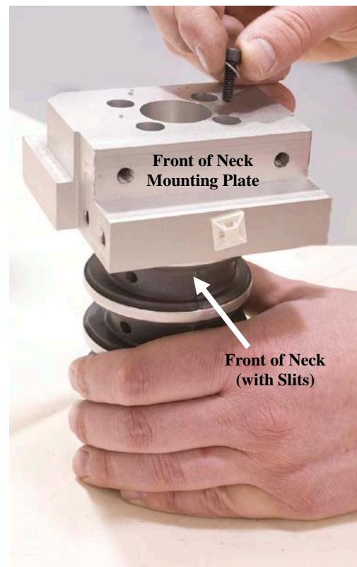
Figure 19. Assemble molded neck to neck mounting plate
