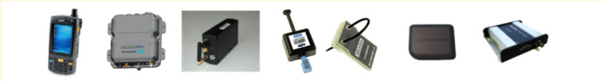
Cell phone, asset monitoring unit, battery, electronic seal, RFID tag, and satellite transmitter used for the Intermodal Cargo and Container Tracking project. Photo source: GlobalTrack, a subsidiary of Orbcomm, Inc.
