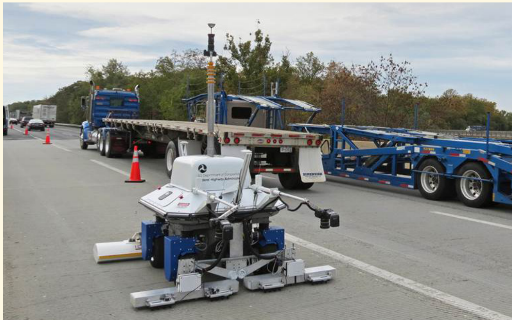
RABIT™ is the first fully automated bridge deck assessment tool to combine multiple nondestructive evaluation technologies that gather a range of condition data and transmit it to a mobile command van in real time. The robot was created by Rutgers' CAIT in partnership with FHWA under the Long-Term Bridge Performance program. ©2013 Nenad Guncuski/Rutgers CAIT.
