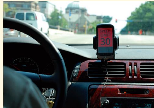
The TDSS uses a smartphone mounted on a vehicle's dashboard to give the driver real-time warnings about speeding and other unsafe behaviors. Photo courtesy of Steve Maturen.
