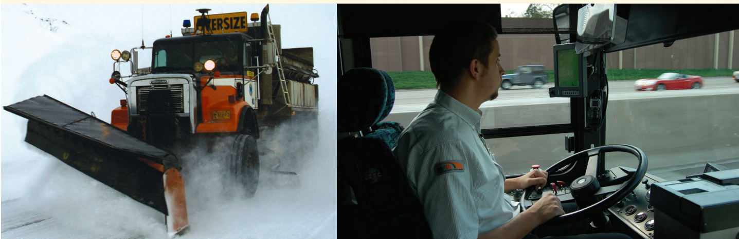
Left: In Alaska, driver-assist technology installed on snowplows helps operators clear Thompson Pass, often in whiteout conditions. Photo courtesy of Alaska Department of Transportation and Public Works. Right: An MVRTA driver views his lane position and other vehicles in the head-up display, part of the driver-assist system. Photo courtesy of Michael McCarthy (ITS Institute).
