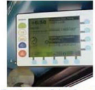
iBus, London, Driver Console (Source: http://www.tfl.gov.uk ) iBus provides next-stop audio-visual announcements, information on points of interest and final destinations, and bus priority
