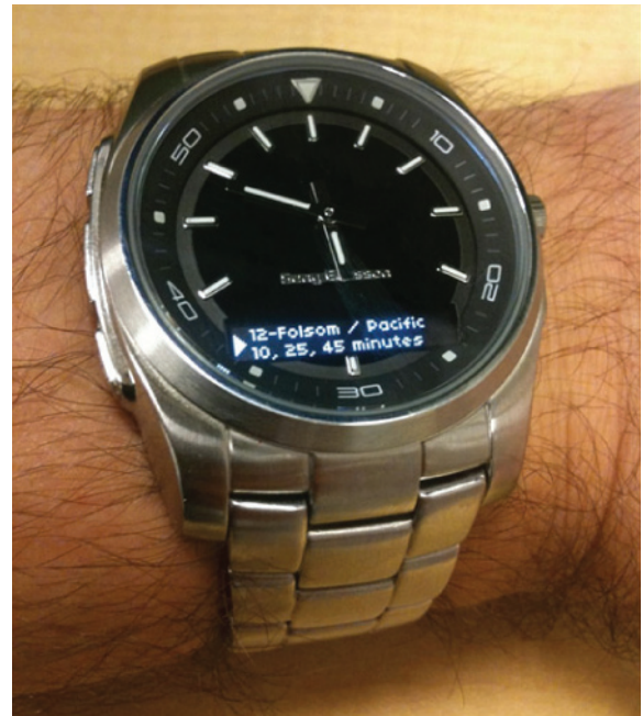
FIGURE 16 Sony Ericsson MBW-150 Bluetooth watch, showing the next few SF Muni Bus arrival times for a nearby stop. [Source: (54).]
