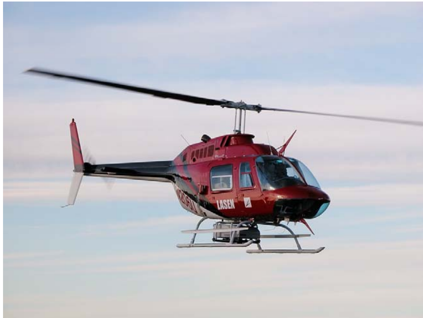
Figure 2. ALPIS-II mounted to a Bell Jet Ranger helicopter.
