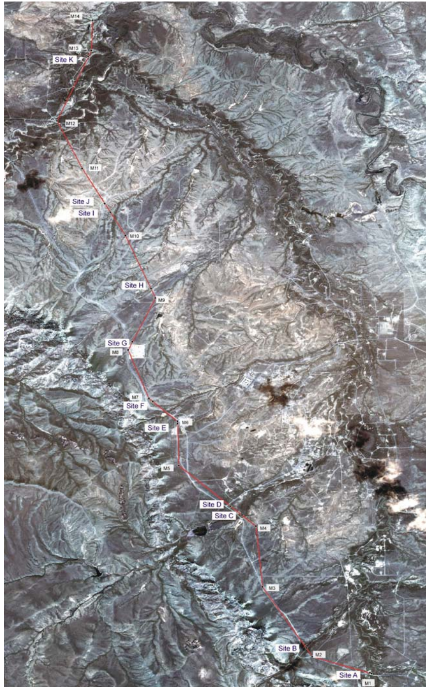
Figure 3. Map of the test site (NPR-3) showing the simulated pipeline route and detected leak sites.
