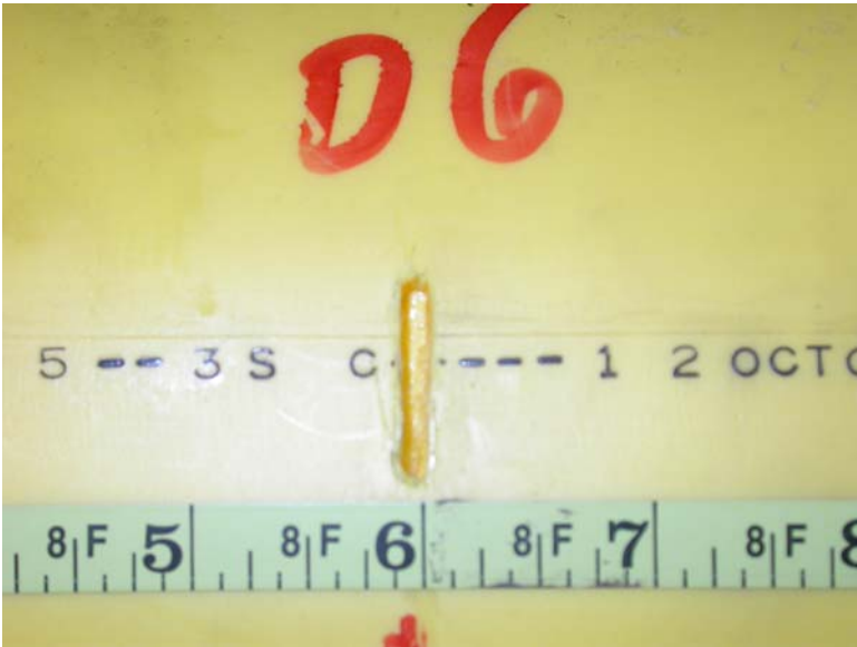
Figure 22. Example Plastic Pipe Defect
