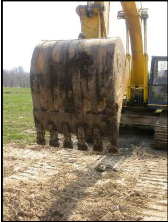
Figure 3-3. Close-Up of Bucket and Teeth from the Kobelco Mark SK200 Track Hoe.
