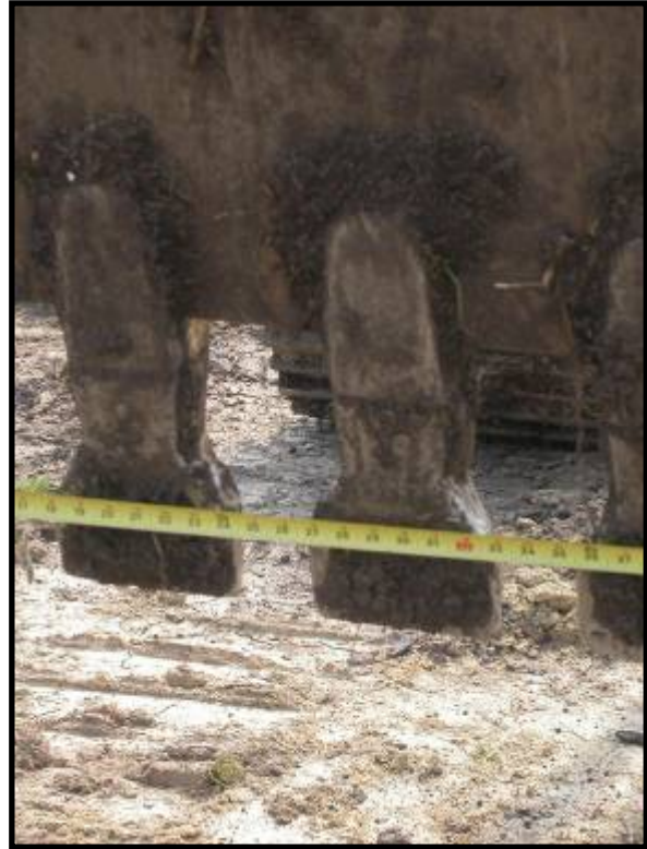
Figure 3-3. Close-Up of Bucket and Teeth from the Kobelco Mark SK200 Track Hoe.
