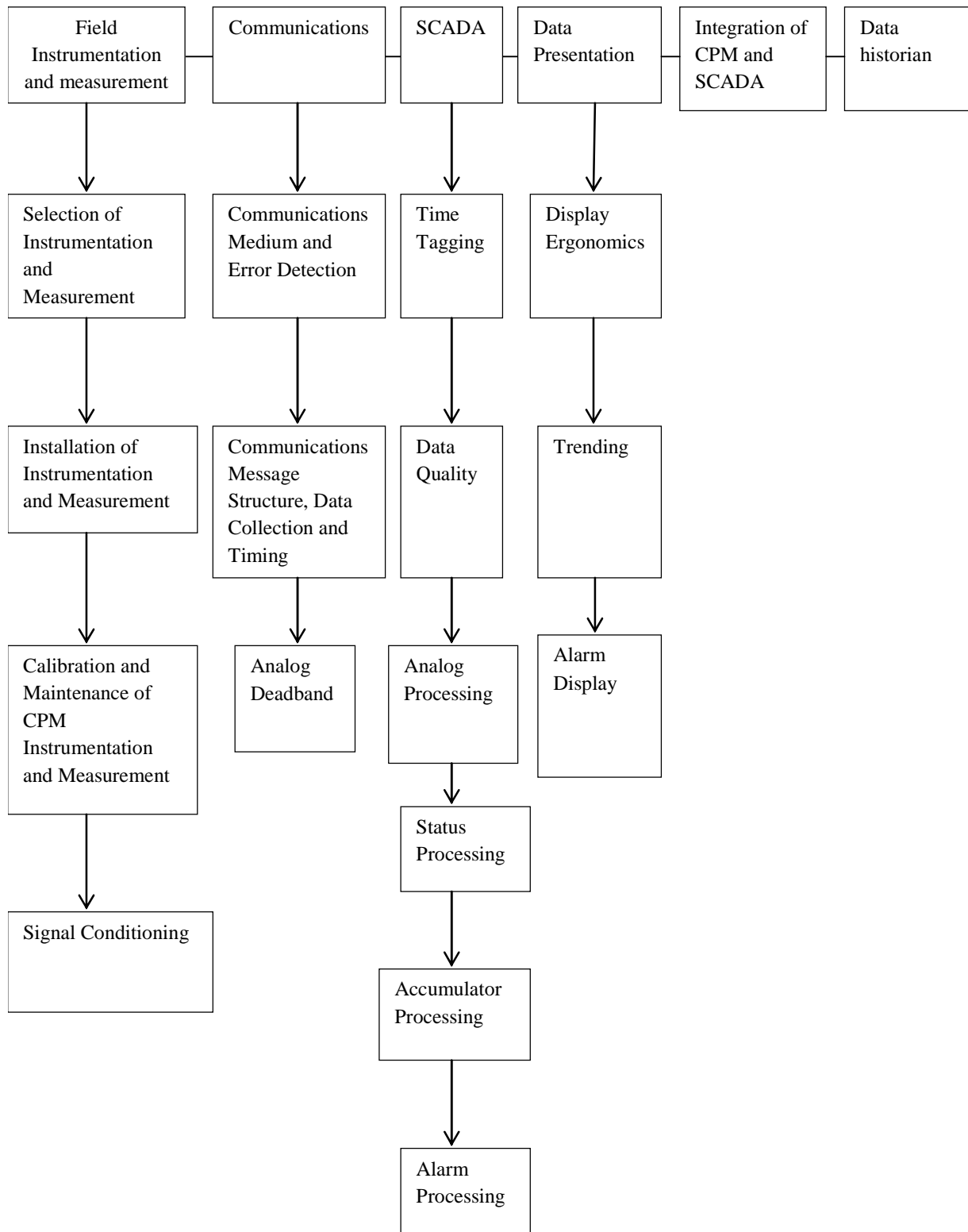
Figure 7.2 Infrastructure Supports for CPM provided by API 1130
