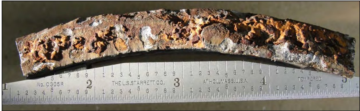
Figure 27. Fracture surface after cleaning with naphtha and Alconox (T014-C-2)
