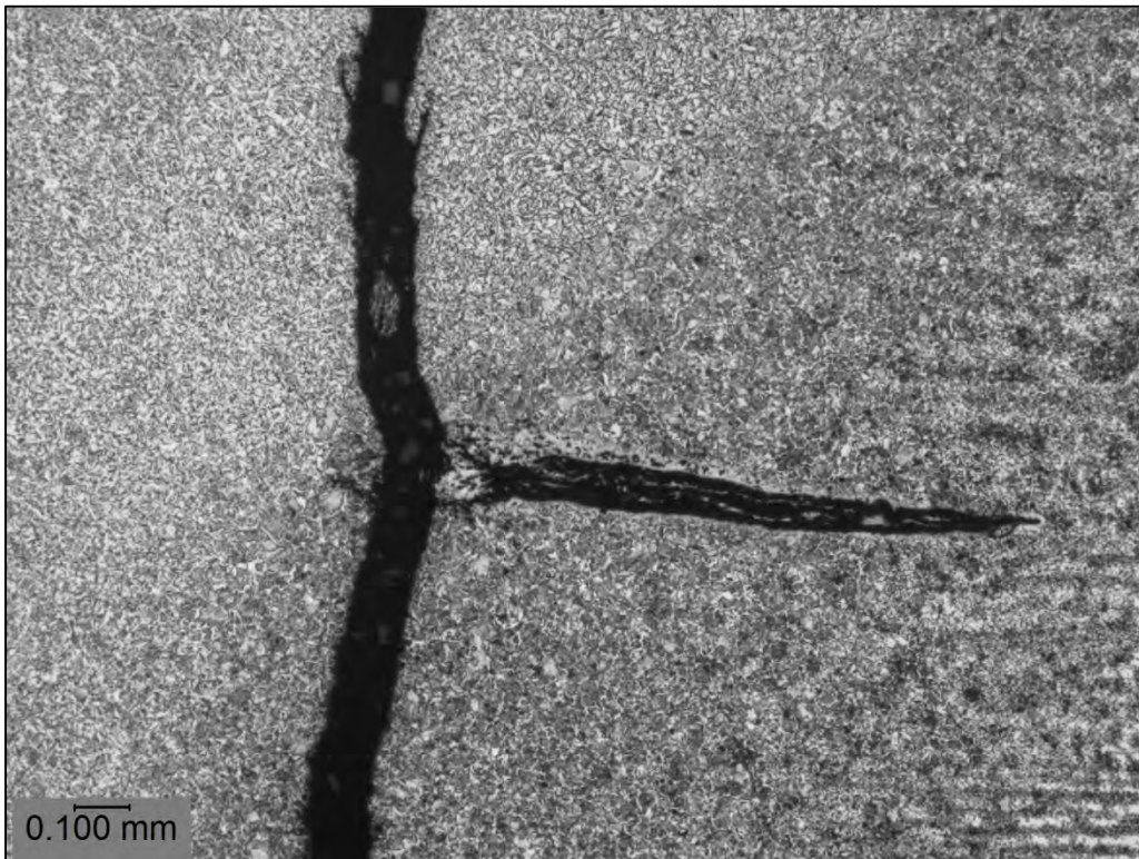
Figure 62. Detail of flaw along crack path in Coupon T026-B-2
