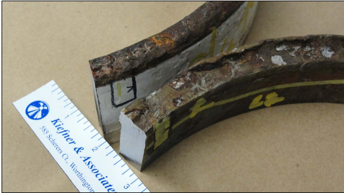
Figure 48. Location of metallographic section in through-wall portion of feature L
