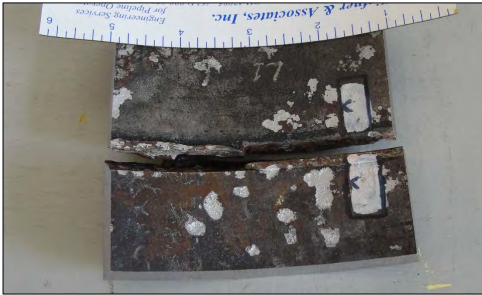
Figure 45. Location of metallographic sections through feature L
