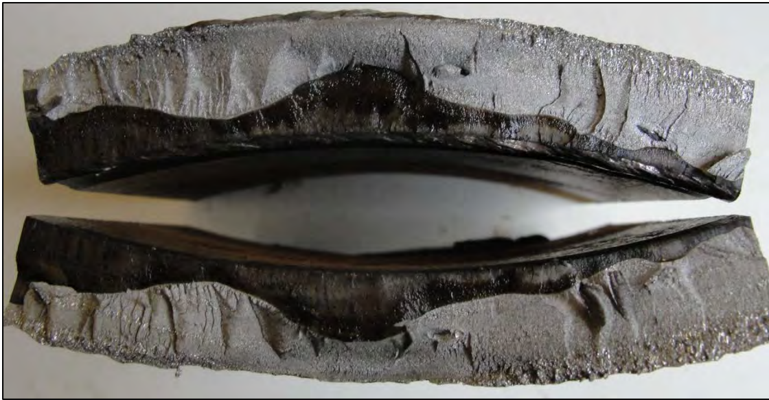
Figure 63. Crack surfaces, Coupon T026-B-2 after breaking open
