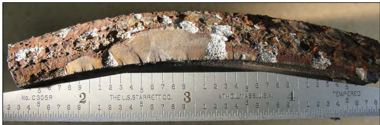
Figure 26. Fracture surface after cleaning with naphtha and Alconox (T014-C-1)
