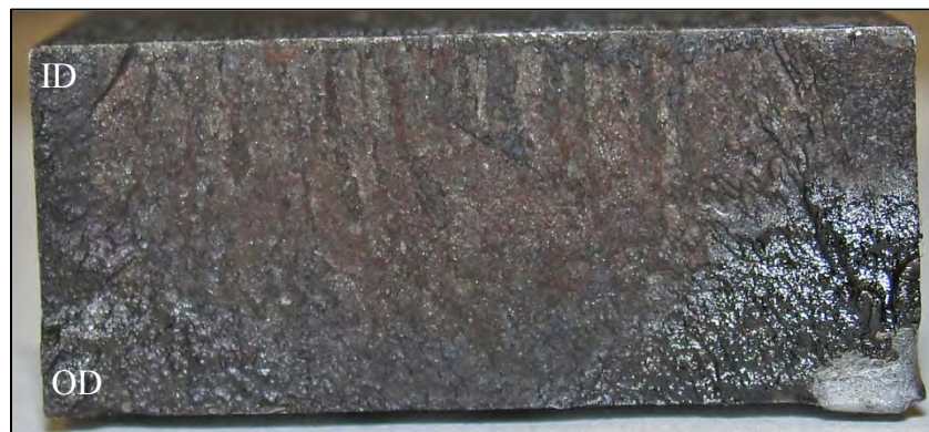
Figure 55. Crack surface of Weld 026 CTOD specimen
