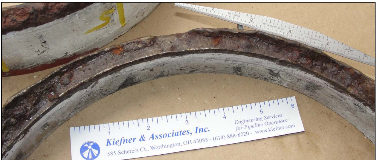
Figure 23. Fracture surface of Pipe 024 showing Feature “L”
