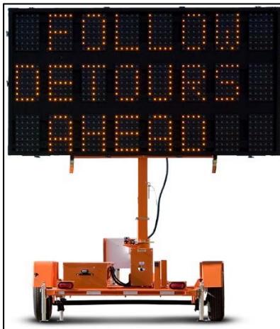
Figure 9-2. Mobile variable message sign (VMS) example.
